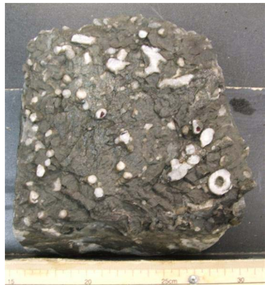
Figure 4. Photograph of a fossil rich dolomite sample after the freeze/thaw test.
