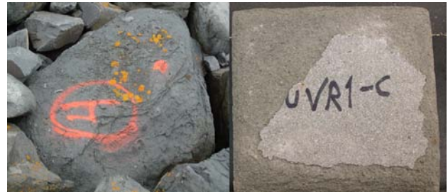
Figure 2. Photographs of disaggregated sandstone from the breakwater (left) and after the freeze/thaw test (right)
