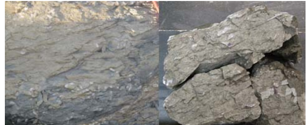
Figure 3. Photographs of disaggregated dolomite located on the wharf (left) and after the freeze/thaw test (right)
