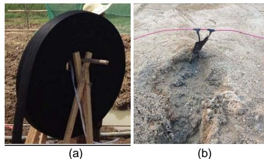
Figure 2. Picture showing: (a) ECWD; (b) connection of two copper wires wrapped in ECWD with the electric wires
