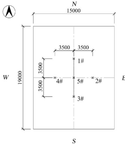
Figure 6 Distribution of the drilling holes after EO (All dimensions are in mm)
