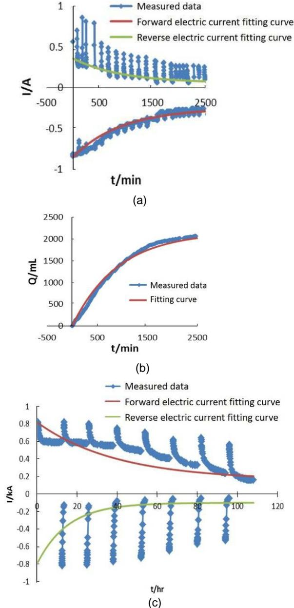
Figure 9 Laboratory and field tests: (a). electric current change with time in the laboratory; (b) accumulative drainage change with time in the laboratory; (c) electric current change with time in the field.
