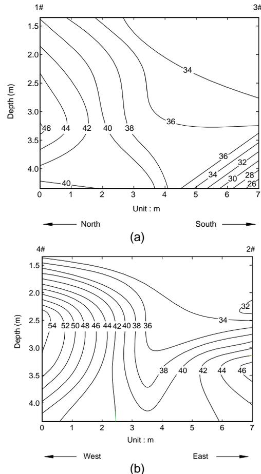
Figure 7 Water content isograms of central cross sections along: (a) east-west direction; (b) south-north direction
