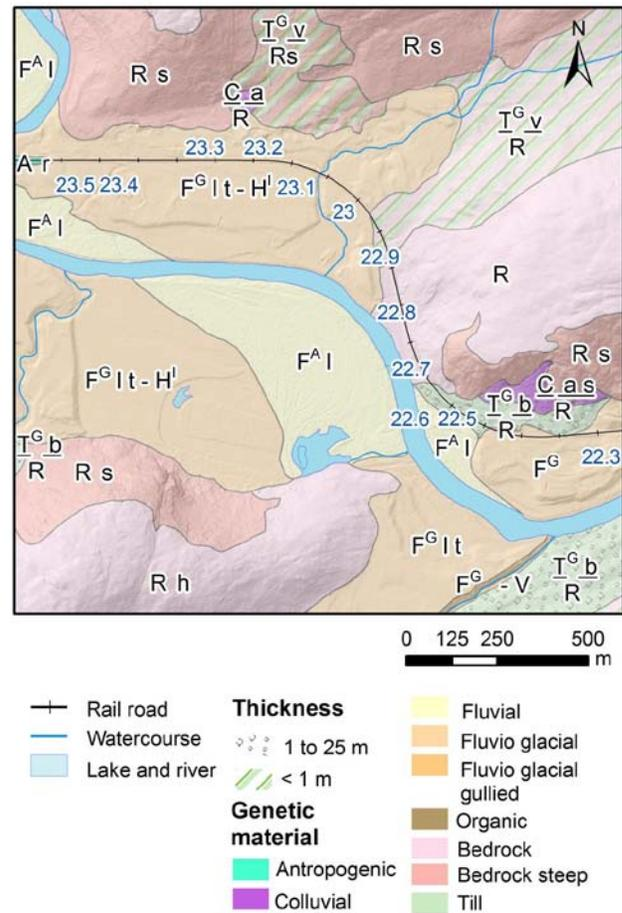
Figure 3. Part of the morpho-structural map along ArcelorMittal's railroad. The lettering on the map is a code that describes the units (Cruden and Thomson 1985). For example, the code  $F^A I$  is a unit where active fluvial deposit is occurring on a leveled topography and  $R_s$  is steep bedrock.
