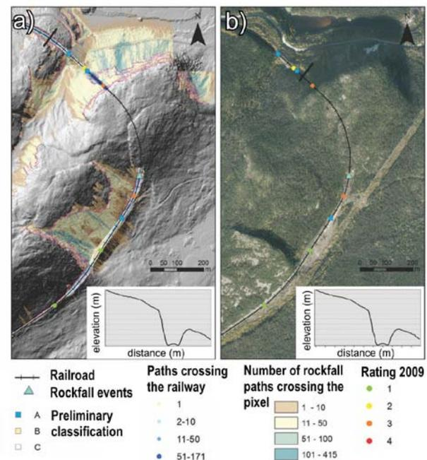
Figure 5. Two scenes in the GIS project used for the preliminary classification of rock slopes. a) Rockfall simulations over the shaded relief image of the topography. b) Same sector as in a), but showing the orthophotos.
