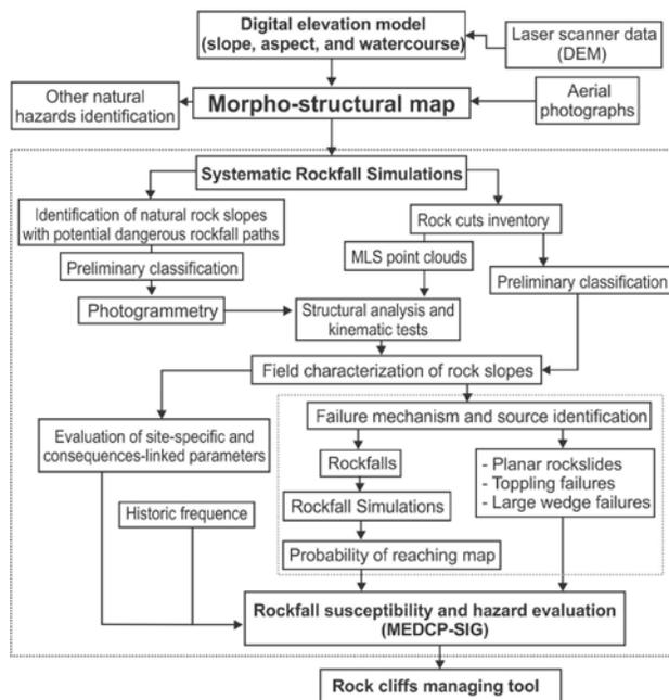
Figure 2. General approach proposed for the development of a rockfall hazard rating system optimizing the use of remote sensing tools. Natural rock cliffs are integrated in the rock slope inventory. The approach focusses on the recognition of failure mechanisms and the identification of rockfall sources.
