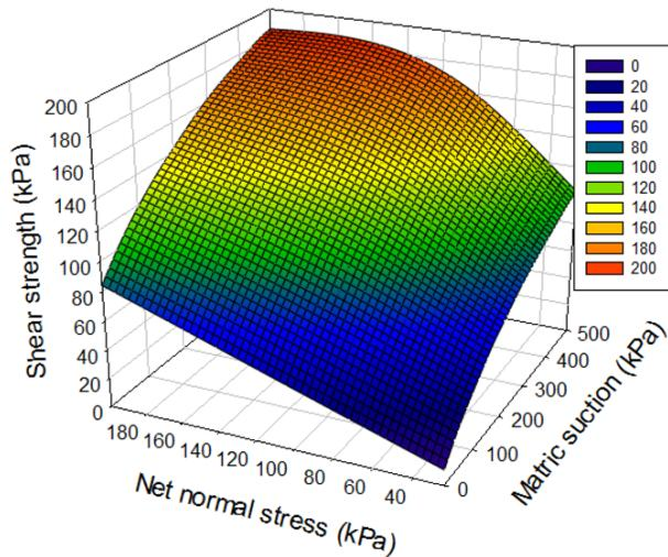
Figure 1. Extended non-linear Mohr-Coulomb failure surface
