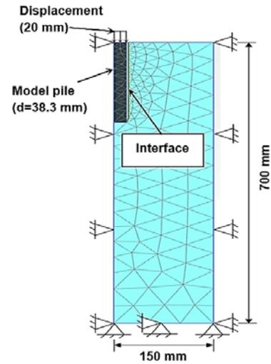
Figure 5. Details of the finite element model.
