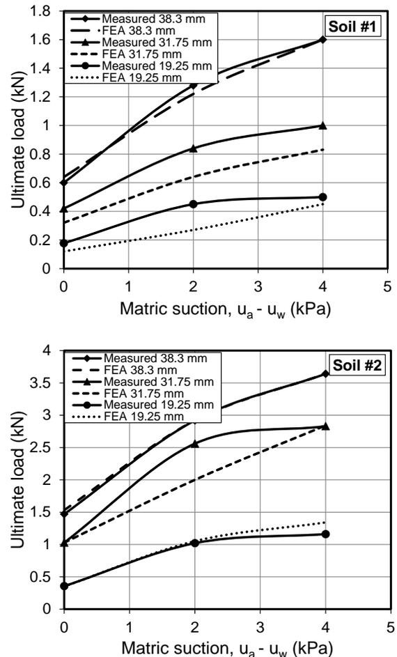
Figure 7. The variation of ultimate load with respect to matric suction,  $u_a - u_w$  for Soil # 1 and Soil # 2.
