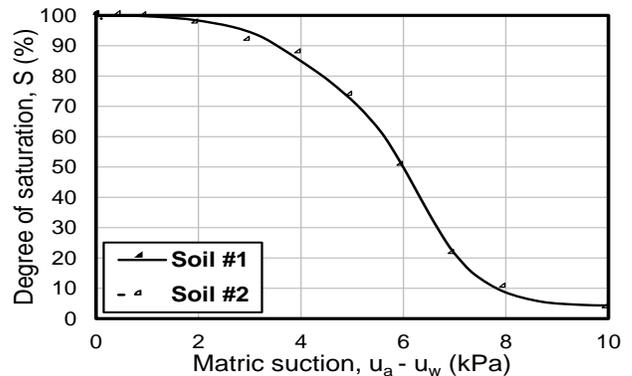
Figure 3. SWCCs for Soil #1 and Soil #2 (from Sheikhtaeri 2014)
