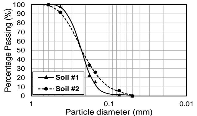
Figure 2. Grain size distribution of the selected soils (from Sheikhtaeri 2014)
