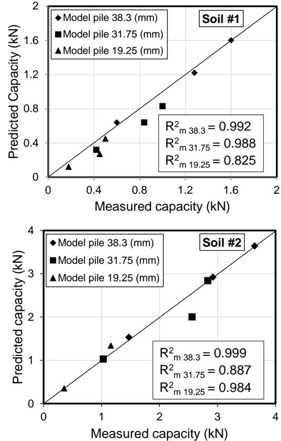
Figure 9. Comparison between the measured and predicted capacities.
