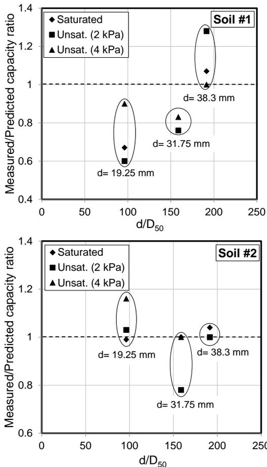
Figure 8. Scale effect of the model pile diameters and the normalized ratio of the measured to predicted capacity.
