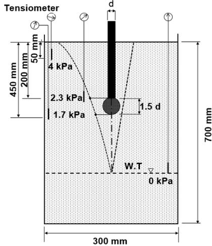
Figure 4. Variation of matric suction with respect to soil depth in the test tank under unsaturated condition of 2 kPa matric suction (modified after Sheikhtaheri 2014)
