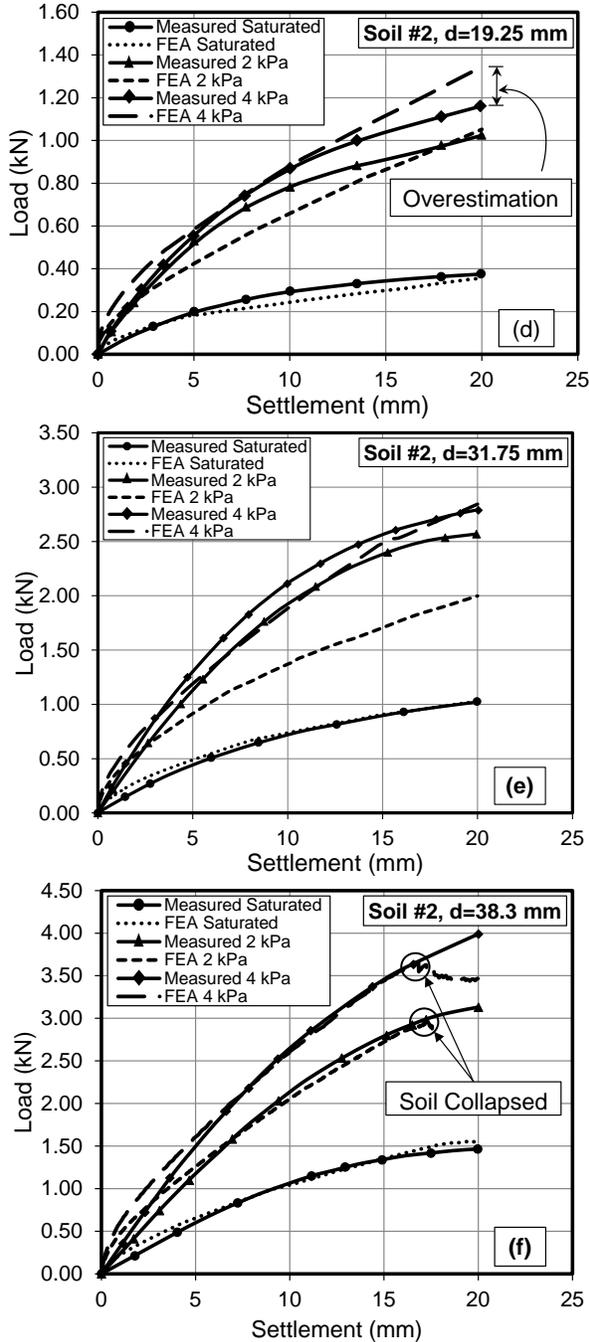
Figure 6. Results of the pile load tests and FEA using PLAXIS 2D under different saturation conditions (i.e., under matric suction of 0 kPa, 2 kPa, and 4 kPa.)
