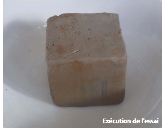
Figure 4a. Sabkha soil sample with 50 mm size before drying
