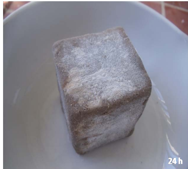
Figure 4b. Sabkha soil sample with 50 mm size after 24 hours of drying
