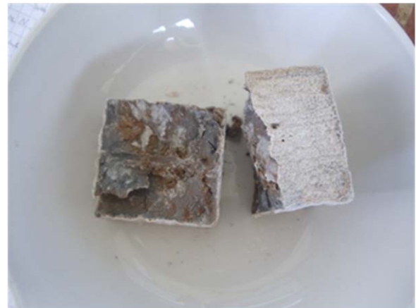
Figure 4c. Sabkha soil sample with 50 mm size after 4 days of drying
