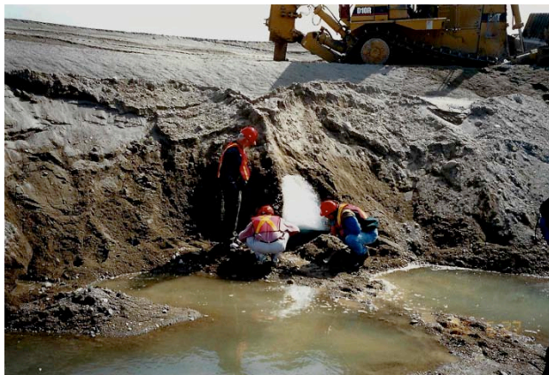
Figure 3. Massive ice exposure at the base of an esker, Ekati Diamond Mine, 1998
