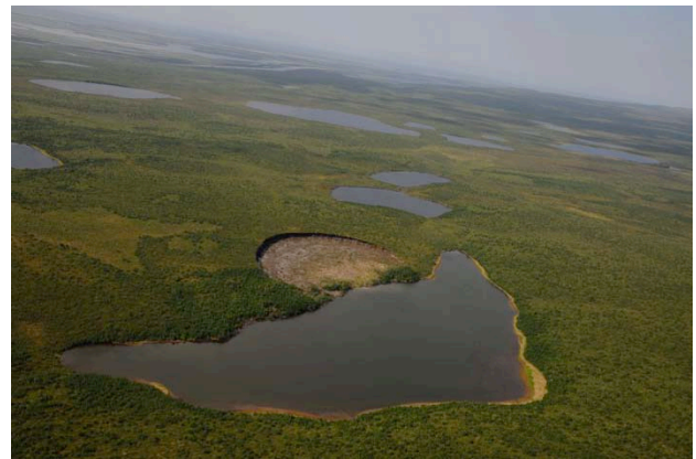
Figure 6. Thermokarst lake with active thaw-flow slide a few km south of ITH route near Inuvik. June, 2012 photo.
