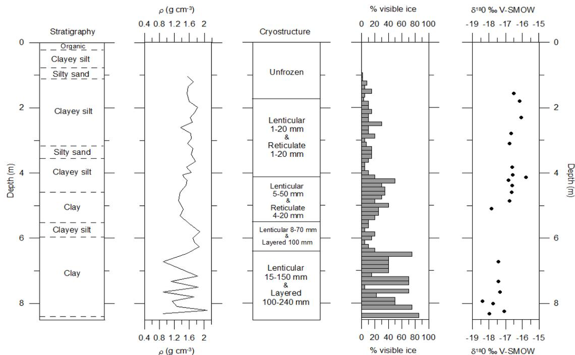
Figure 3. Stratigraphy, frozen bulk density ( $\rho$ ), cryostructures, visible ice, and  $\delta^{18}\text{O}$  values at BH04 (top of feature is approximately 4 m above the surface of the peatland).
