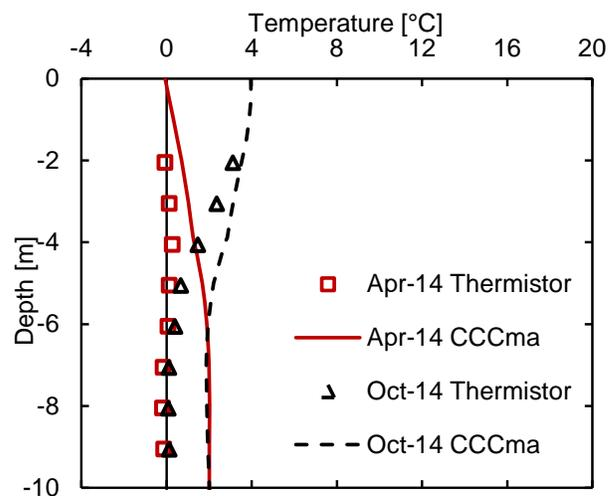
Figure 5: Comparison between the measured (symbol) and modelled (line) ground temperature data at the shoulder in April and October of 2014.
