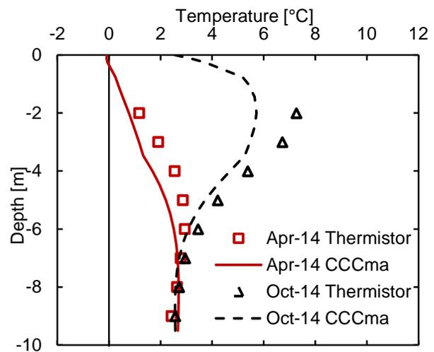
Figure 4: Comparison between the measured (symbol) and modelled (line) ground temperature data at the toe in April and October of 2014.
