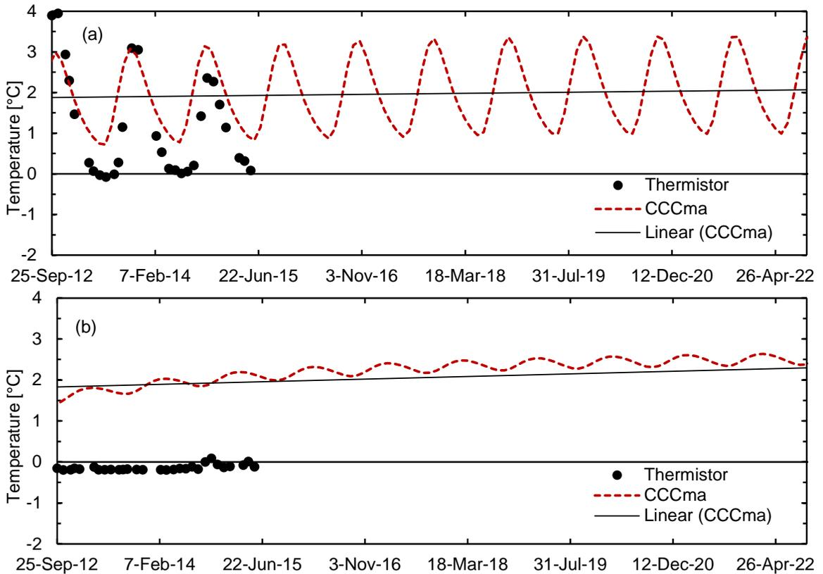
Figure 7: Temperature versus time for 10 years at (a) 3 m and (b) 8 m below the shoulder of the embankment
