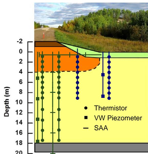
Figure 2: Instrumentation installed. (Note: Blue indicates instrumentation installed in 2008. Green indicates instrumentation installed in 2012). (Flynn et al., 2013).
