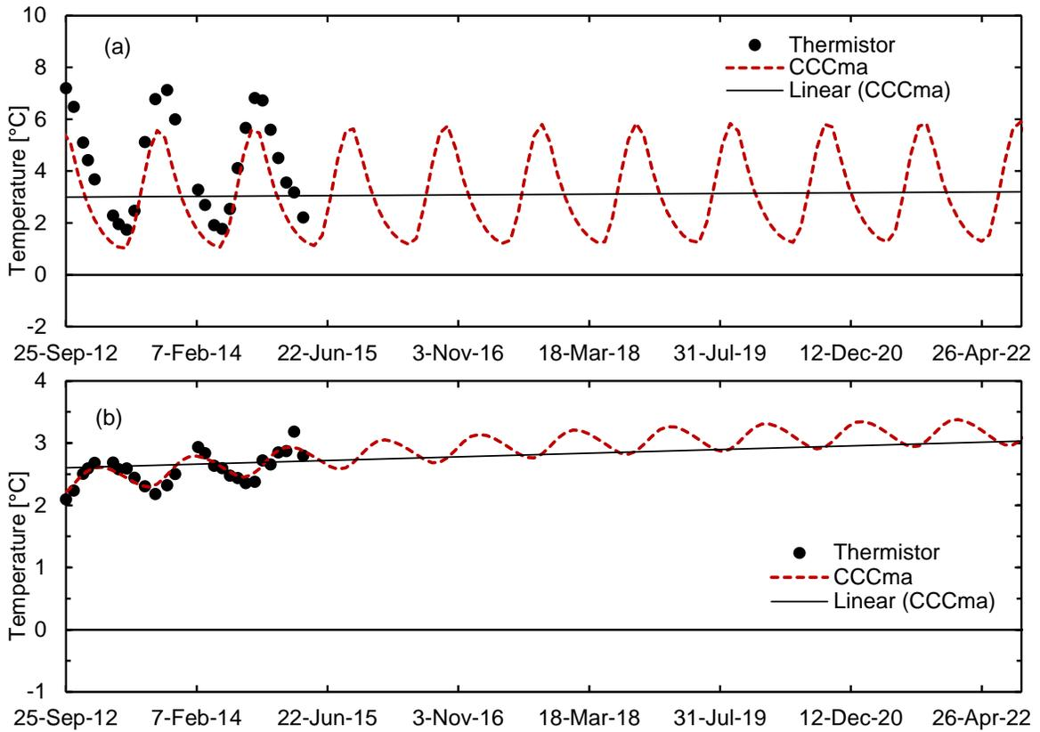
Figure 6: : Temperature versus time for 10 years at (a) 3 m and (b) 8 m below the toe of the embankment
