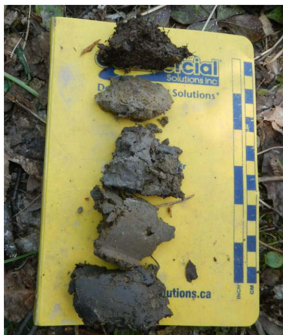
Figure 5. Soil and surficial material samples collected from different depths to two metres. Note the difference in colour, structure and texture and how they change with depth. Each layer will have different characteristics that play into soil handling plans, especially on pipelines.
