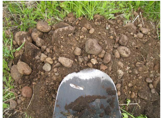
Figure 1. Glaciofluvial deposit with sandy loam texture but high coarse fragments limits the reclamation suitability. Geotechnical drill logs can provide this type of information for the entire depth of the drill core.
