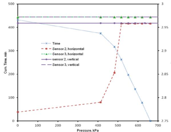
Figure 11 Sensor response to decreasing pressure
