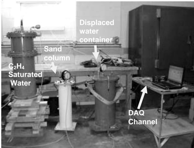
Figure 7 Lab setup of sand column test
