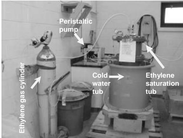
Figure 3 Lab setup of water saturation with ethylene.
