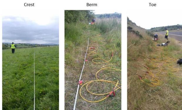
Figure 3: Picture showing the layout of the geophones at the crest, berm and toe of the Loughbrickland cutting
