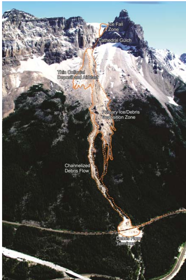
Figure 2. Overview of Cathedral Gulch showing the debris flow and two of the three CP tracks and the TransCanada Highway. The glacier is just visible above the Gulch.
