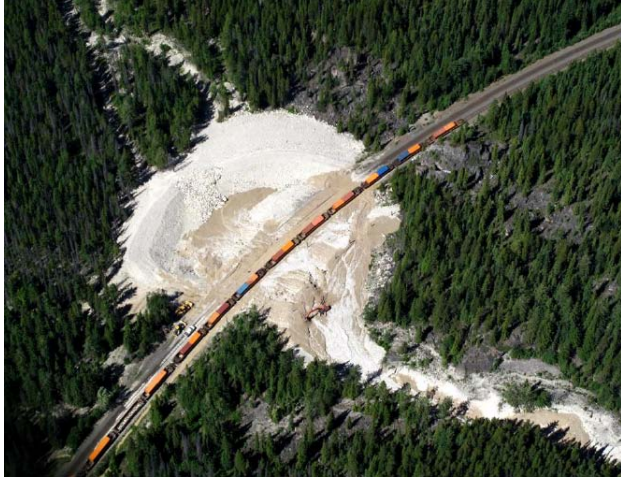
Figure 5. Sediment basins above and below the CP tracks. The first basin and the tracks were overrun.
