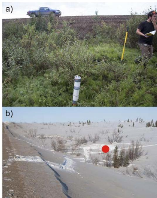
Figure 3. Site TST2 near the highway embankment showing a) the thermistor cable installation and embankment in summer, and b) snow accumulation in winter. Note that many of the tall shrubs are covered by deep snow in winter. The red dot indicates the location of the thermistor cable.
