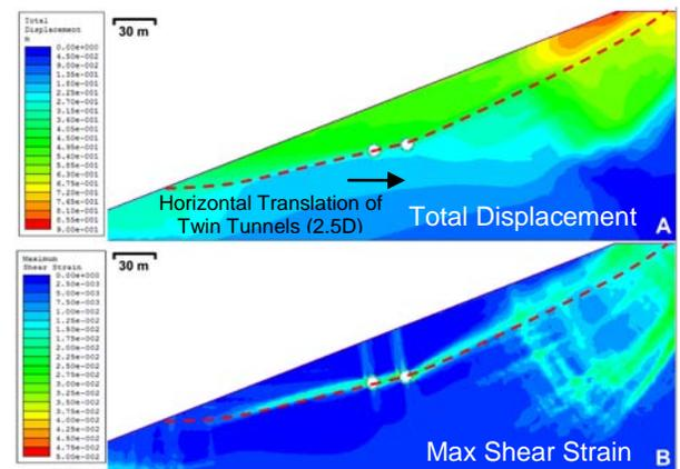
Fig 8. (A) Total displacement and (B) maximum shear strain contours of the slope after the excavation of the tunnels. The tunnels have been translated horizontally a distance of 2.5D relative to their initial location.
