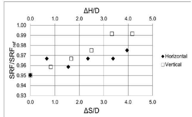
Fig 12. The influence of the horizontal and vertical translation of the tunnels on the SRF values and the safety factor of the slope. D is the diameter of the tunnels,  $\Delta S$  the relative horizontal translation of the tunnels to the initial tunnel location and  $\Delta H$  the relative vertical translation.
