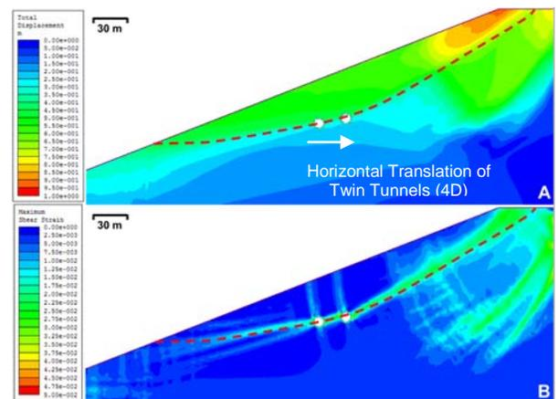
Fig 9. (A) Total displacement and (B) maximum shear strain contours of the slope after the excavation of the tunnels. The tunnels have been translated horizontally a distance of 4D relative to their initial location.
