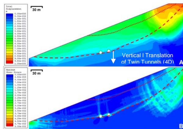
Fig 11. (A) Total displacement and (B) maximum shear strain contours of the slope after the excavation of the tunnels. The tunnels have been translated vertically a distance of 4D relative to their initial location.
