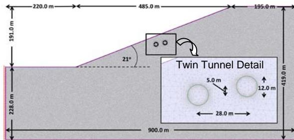
Fig 5. Numerical model configuration for the S3 Tunnel of the Egnatia Odos Project developed in Phase2
