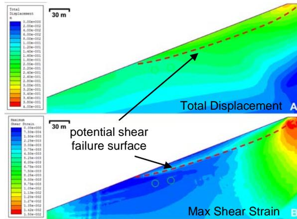
Fig 6. (A) Total displacement and (B) maximum shear strain contours of the slope prior to the excavation of the tunnels
