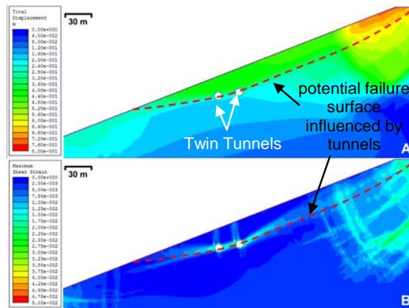
Fig 7. (A) Total displacement and (B) maximum shear strain contours of the slope after the excavation of the tunnels. The tunnel location relative to the slope was determined based on the actual design specifications of the project.
