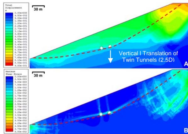
Fig 10. (A) Total displacement and (B) maximum shear strain contours of the slope after the excavation of the tunnels. The tunnels have been translated vertically a distance of 2.5D relative to their initial location.
