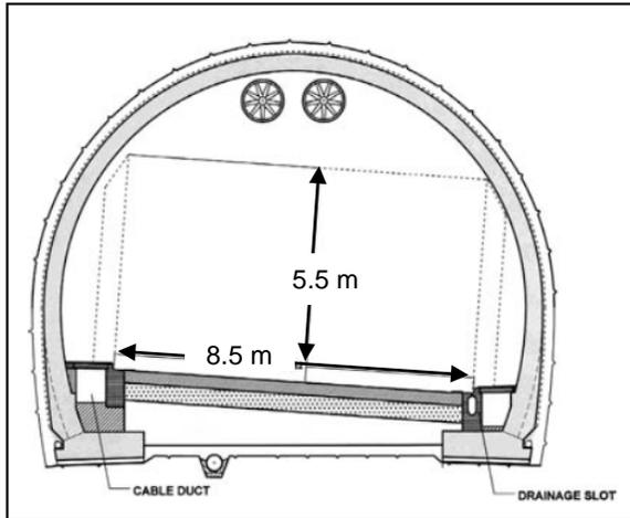
Fig. 2. Eganatia Odos highway tunnel; typical cross-section (Aggitalis et al., 2004)
