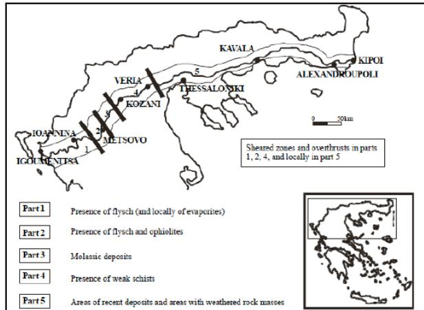
Fig. 1. Alignment of the Egnatia Highway showing spatial setting of the major geological sections along with unfavourable geotechnical characteristics (Marinos & Hoek, 2001).
