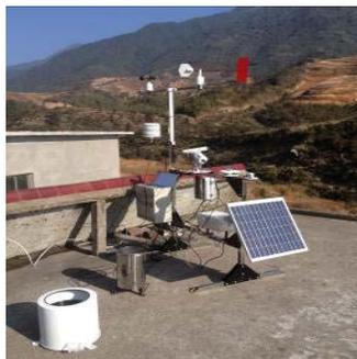
Fig.3 Automatic meteorological monitoring station
