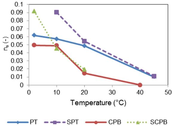
Figure 7. Effect of temperature on the Sisko viscosity index  $n_s$  for PT, SPT, CPB and SCPB mixtures
