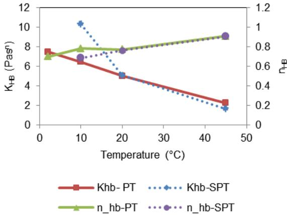
Figure 3. Variation in the consistency index and flow index as a function of temperature for PT and SPT
