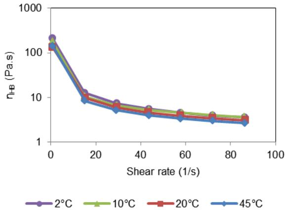
Figure 5. Viscosity curves of PT conditioned at 2, 10, 20 and 40°C
