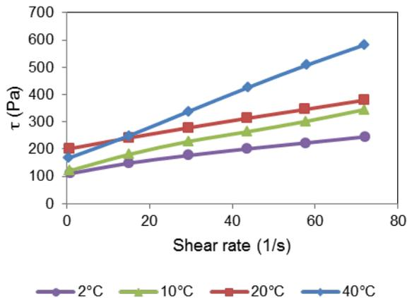
Figure 2. Flow curves for CPB samples conditioned at 2, 10, 20 and 40°C
