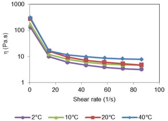
Figure 4. Viscosity curves of CPB as a function of the shear rate at temperature of 2, 10, 20 and 40°C
