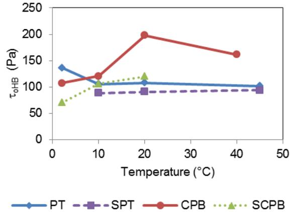
Figure 1. Variation in the yield stress as a function of temperature for PT, SPT, CPB and SCPB samples
