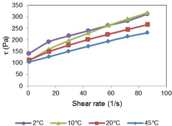
Figure 1. Flow curves for uncemented paste tailings (PT) conditioned at 2, 10, 20 and 45°C
