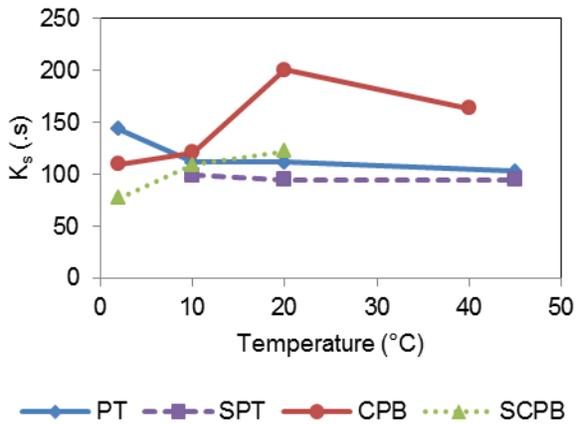
Figure 8. Variation in the Sisko consistency index  $K_s$  as a function of temperature for PT, SPT, CPB and SCPB mixtures
