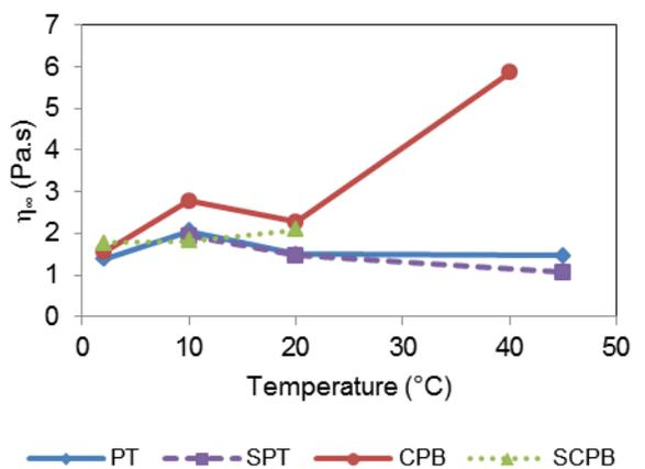
Figure 6. Effect of temperature on the viscosity at high shear rate for PT, SPT, CPB and SCPB
