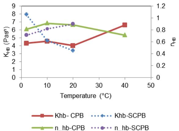
Figure 2. Variation in the consistency index and flow index as a function of temperature for CPB and SCPB
