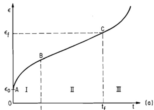
Figure 1. The three stages of creep behavior (Ladanyi 1972).
