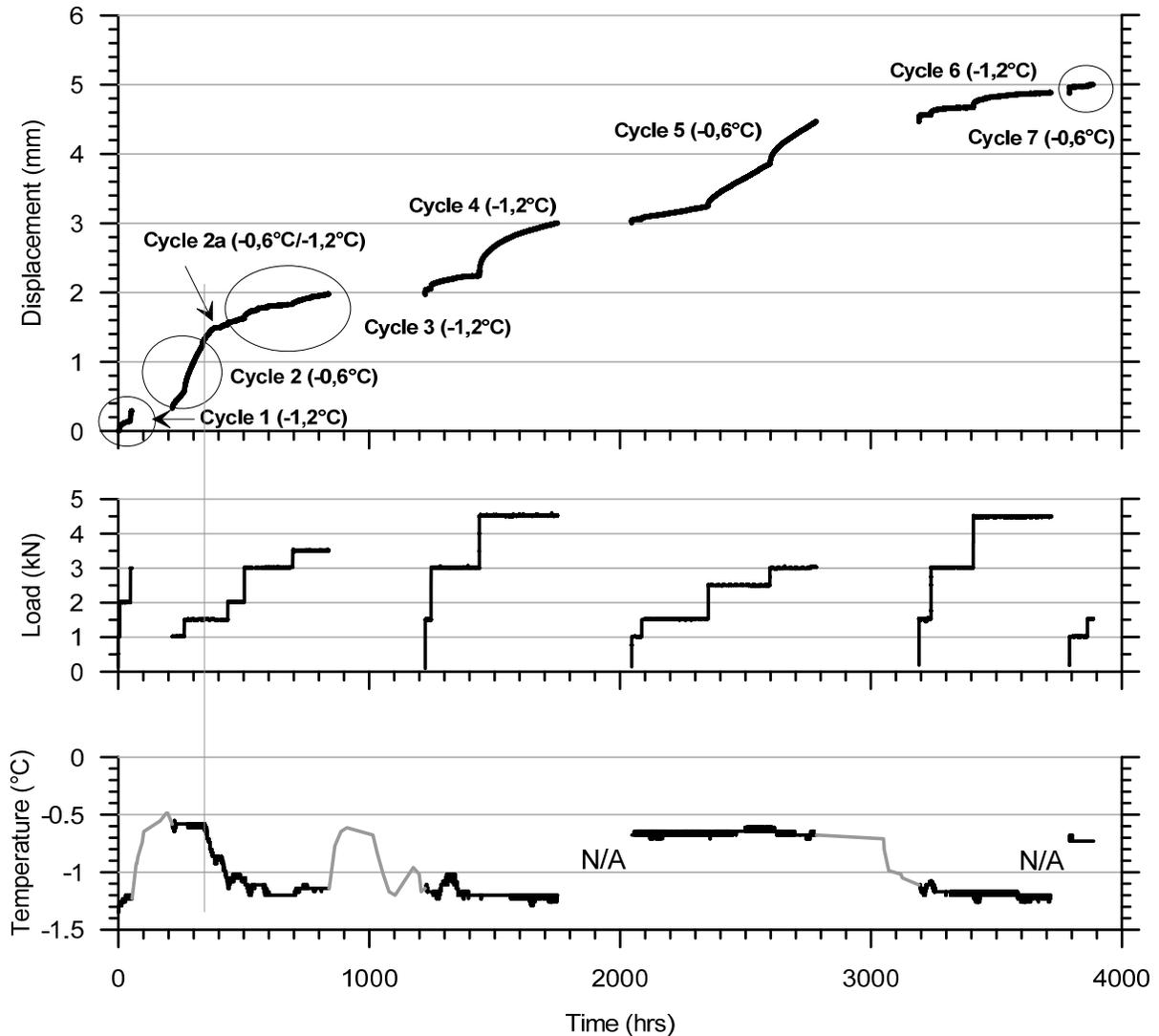
Figure 6. Summary of the creep tests on the enlarged-base anchor.
