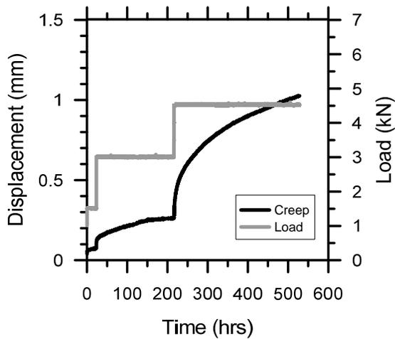
Figure 8. Typical creep behavior of the enlarged-base anchor at a temperature of  $-1.2^{\circ}\text{C}$  (cycle 4).
