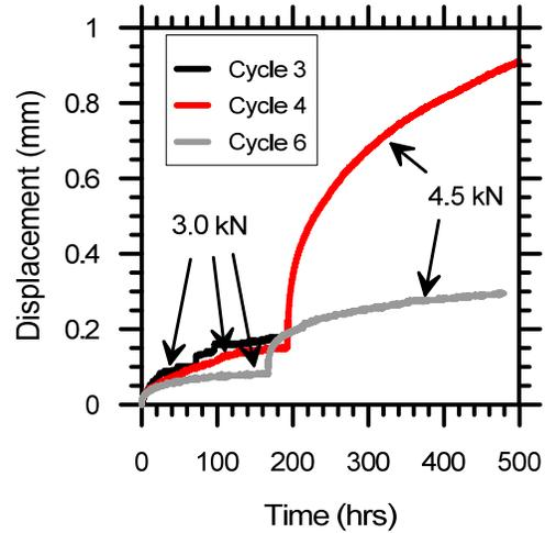
Figure 10. Effect of different loading cycle on creep behavior; coned-base anchor, temperature of  $-1,2^{\circ}\text{C}$ .
