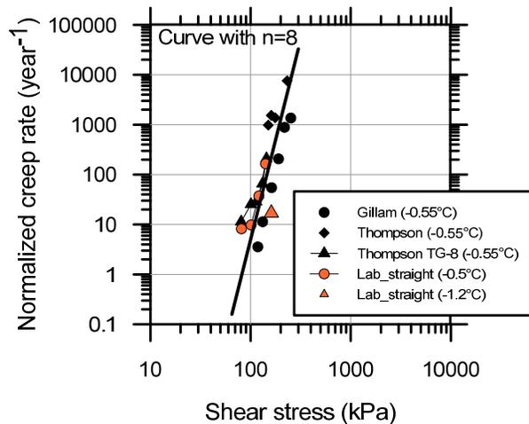
Figure 12. Creep behavior on straight anchor; comparison between data from Johnston and Ladanyi (1972) and our study.
