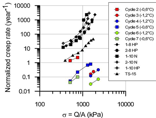
Figure 13. Creep behavior of screwed anchors from Johnston and Ladanyi (1974) and the enlarged-base anchor of our study.
