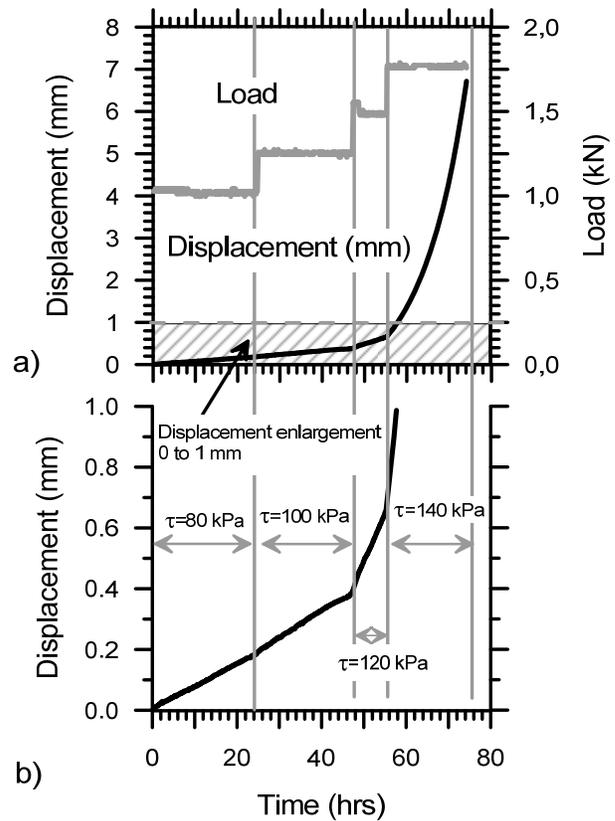
Figure 4. Creep test results for the straight anchor at -0.5°C.
