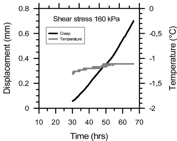
Figure 3. Creep test results for the straight anchor at a temperature of -1.3/1.1°C.
