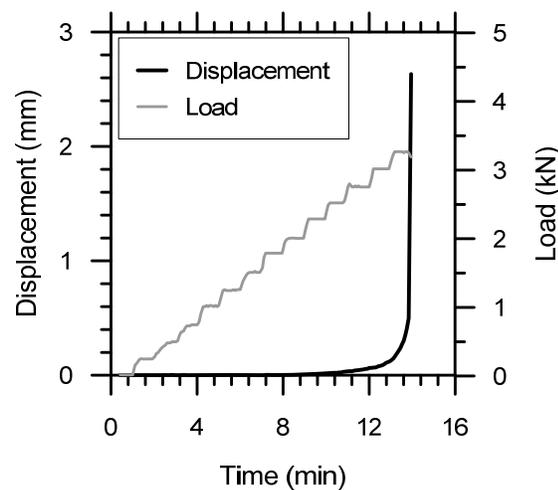
Figure 5. Pullout test on the straight anchor at a temperature of  $-0.5^{\circ}\text{C}$ .
