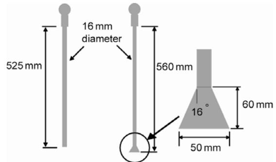
Figure 2. Geometry of the tested anchors.
