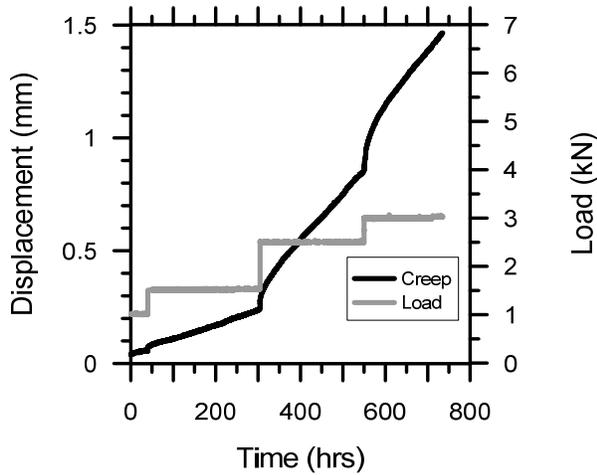
Figure 7. Typical creep behavior of the enlarged-base anchor at a temperature of  $-0.6^{\circ}\text{C}$  (cycle 5).
