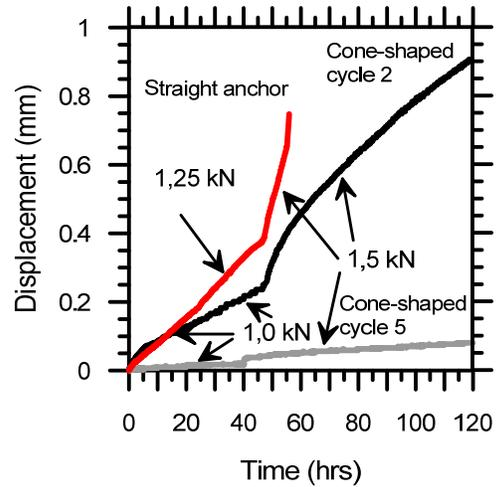
Figure 9. Effect of different loading cycles on the creep behaviour of the cone-based anchor at a temperature of  $-0.6^{\circ}\text{C}$ .
