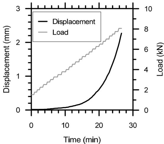
Figure 11. Pullout test on enlarged-base anchor at  $-0.6^{\circ}\text{C}$ .
