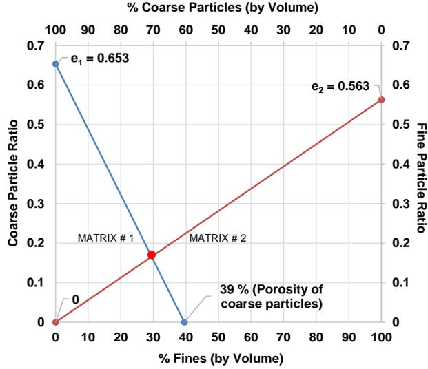
Figure 6. Theoretical variation of minimum void ratio in binary packing with % fines.
