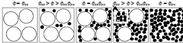
Figure 4. Dispersed mixing mode of coarse and fine grains (Dvorkin and Gutierrez, 2002).
