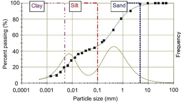
Figure 2. Arithmetic probability density function of a gap graded soil (Fredlund et al., 2000).
