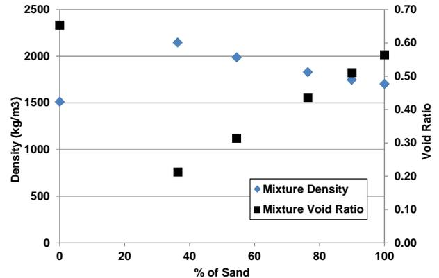
Figure 5. Mixture void ratios and densities with respect to sand content.
