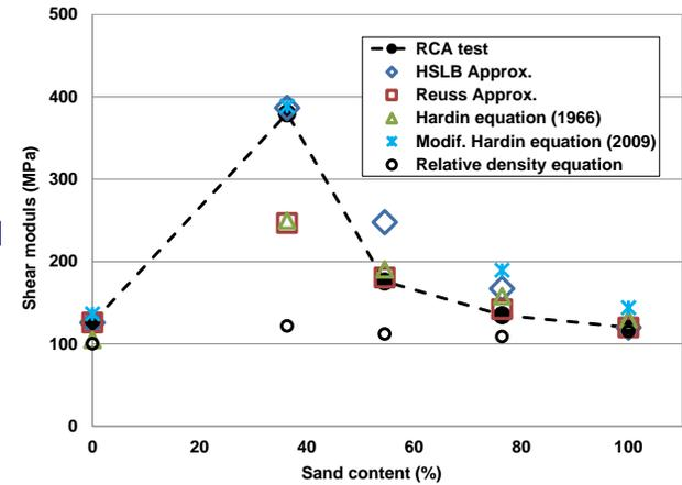
Figure 7. Measured and estimated values of  $G_{max}$  at 120 kPa.
