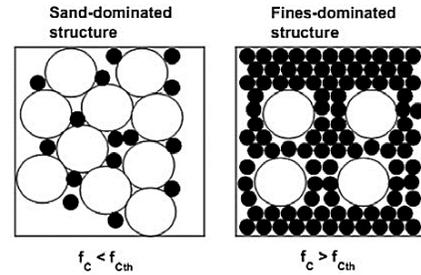
Figure 3. Configuration of Sand with Fines (Benahmed, 2014).
