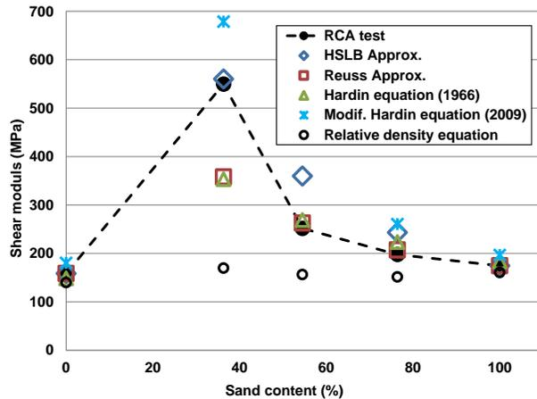
Figure 8. Measured and estimated values of  $G_{max}$  at 240 kPa.
