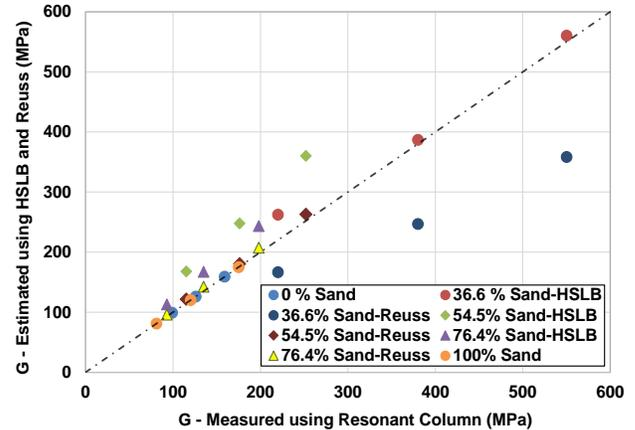
Figure 9. Comparison of estimated vs. measured values of  $G_{max}$ .
