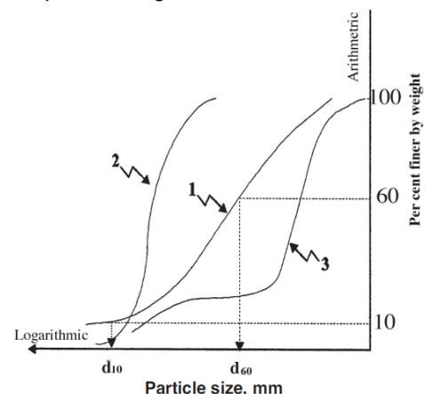
Figure 1. Characteristic particle size gradation curves (Senyur, 1998).
