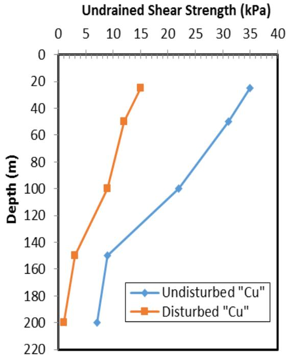
Figure 2. Undisturbed and disturbed shear strength profiles for Leda clay
