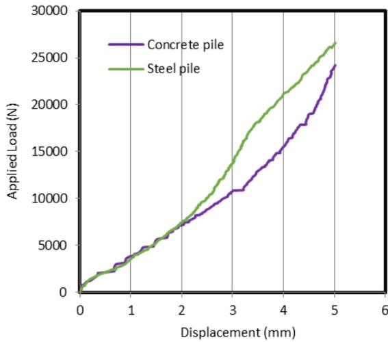
Figure 7. Load-displacement curves for piles in frozen Leda clay.
