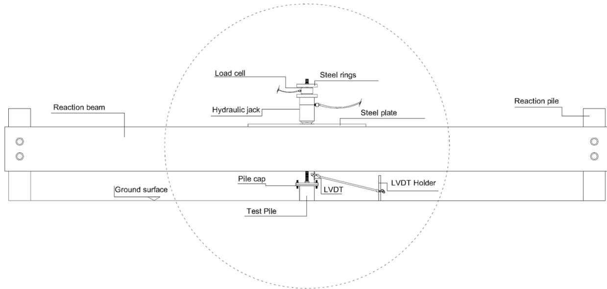
Figure 5. Pile load test instrumentation and setup
