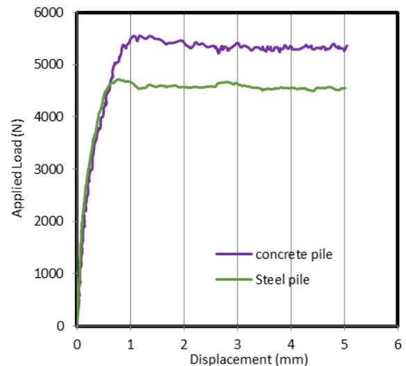
Figure 6. Load-displacement curves for piles in unfrozen Leda clay
