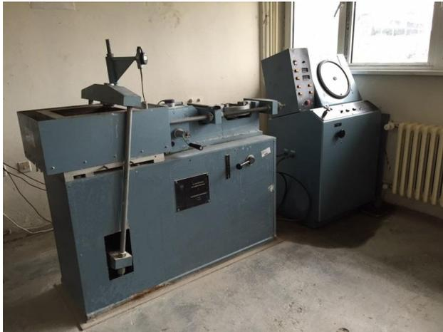
Figure 4. Direct shear box (300 mm x 300 mm) (from Tanriseven 2012)
