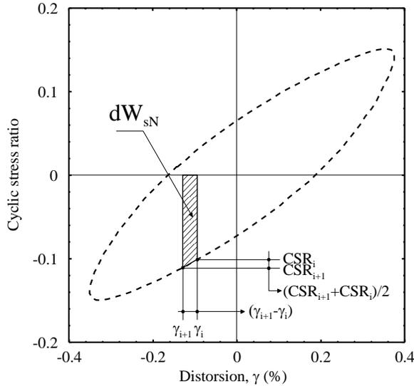
Figure 3. Dissipated energy per unit volume for a soil sample in cyclic  $T_xSS$  test determined by integrating area bound by stress-strain hysteresis loops
