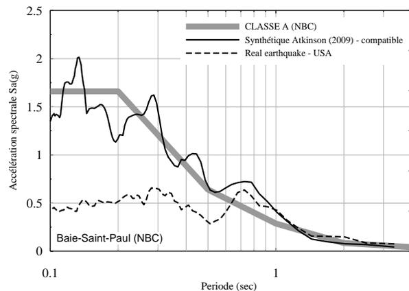
Fig. 11. NBCC 2005 spectrum for Baie-Saint-Paul site on NBCC (A) compared to compatible (Atkinson 2009) and incompatible records
