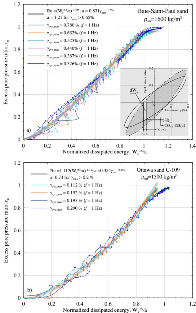
Figure 4.  $r_u$ - $W_s$  for soil samples tested in the cyclic  $T_xSS$ : (a) Baie-Saint-Paul sand; (b) Ottawa sand C-109
