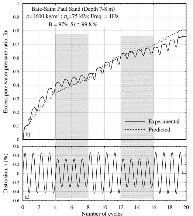
Fig. 6. Comparison of measured versus predicted excess pore pressure ratios for irregular loading 1: Baie-Saint Paul sand.
