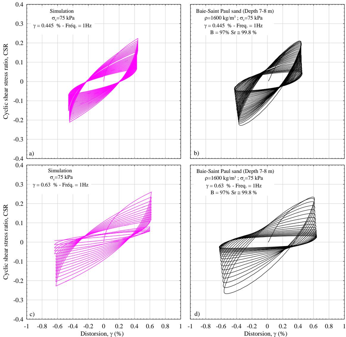
Fig. 10. Comparison between measured and computed CSR- $\gamma_{cyc}$  loops: (a), (b)  $\gamma_{cyc} = 0.445\%$  and (c), (d)  $\gamma_{cyc} = 0.63\%$
