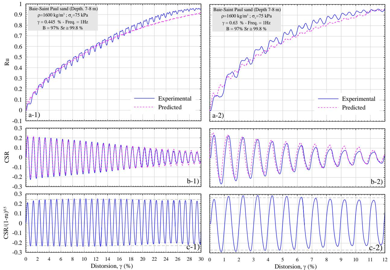
Fig. 9. Comparison of measured versus predicted Baie-Saint-Paul sand cyclic response tested at  $\gamma_{cyc}$  of 0.445% and 0.63%: (a) excess pore pressure; (b) CSR; and (c)  $CSR/(1-r_u)^{0.5}$
