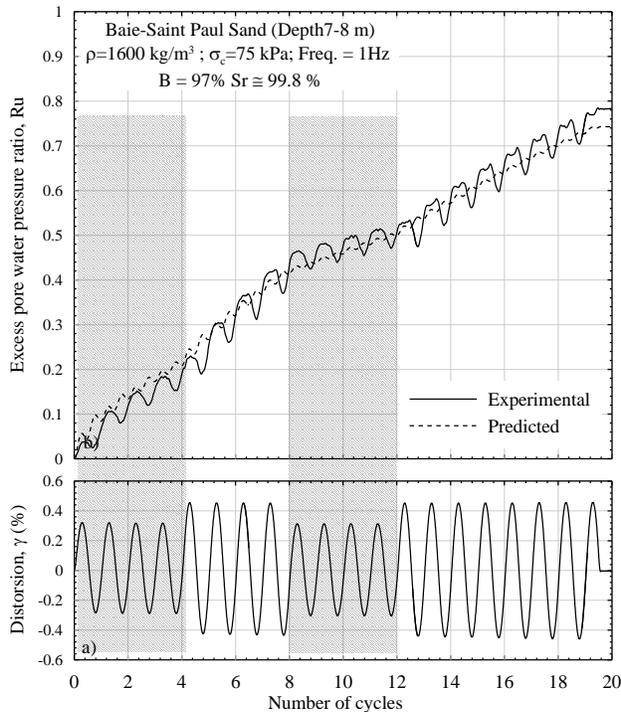
Fig. 7. Comparison of measured versus predicted excess pore pressure ratios for irregular loading 2: Baie-Saint Paul sand
