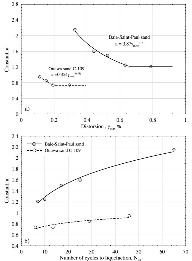
Figure 5. Calibration parameter versus: (a) distortion; (b) number of cycles to liquefaction
