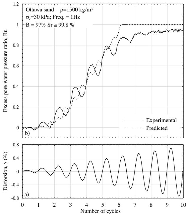
Fig. 8. Comparison of measured versus predicted excess pore pressure ratios: Ottawa sand
