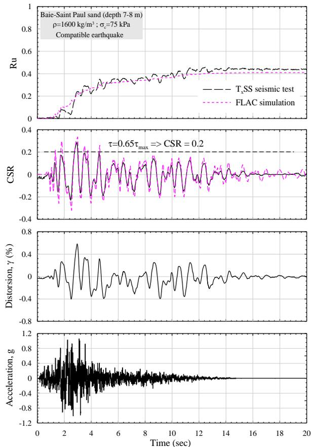
Fig. 12. Measured and computed response of Baie-Saint-Paul sand to a compatible record with NBCC 2005 spectrum
