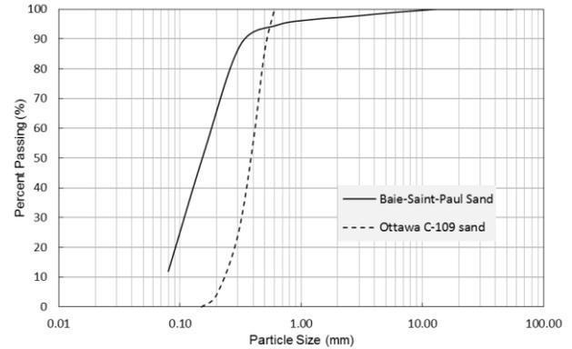
Figure 1. Grain size distribution curves of the used sands
