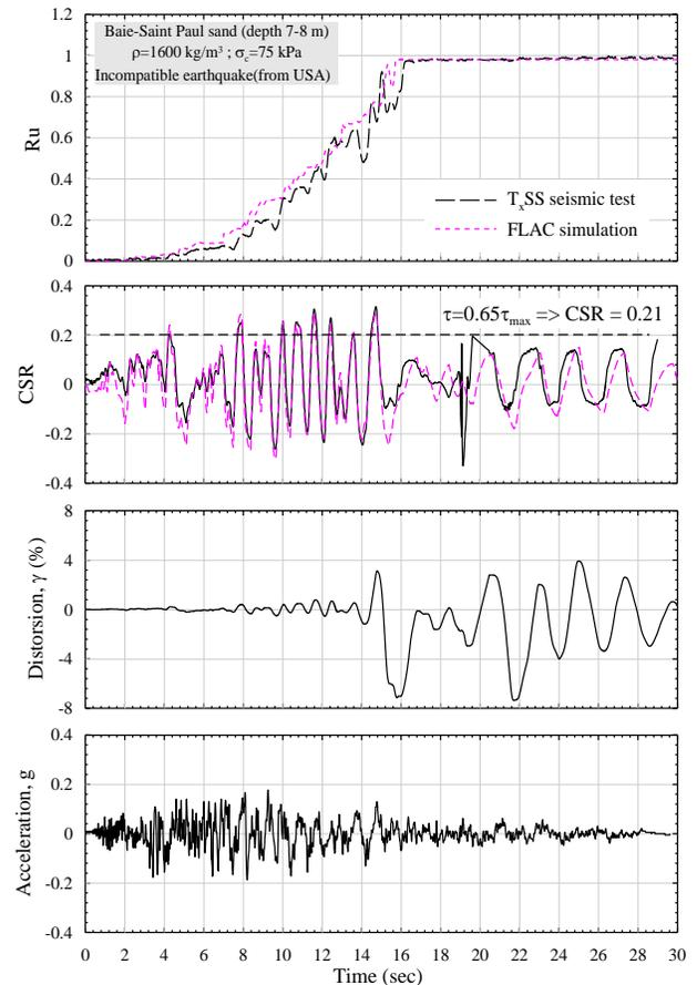
Fig. 13. Measured and computed response of Baie-Saint-Paul sand to an incompatible record with NBCC 2005 spectrum
