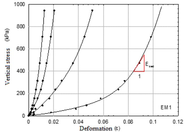
Figure 1. Vertical stress-vertical strain curve for EM1
