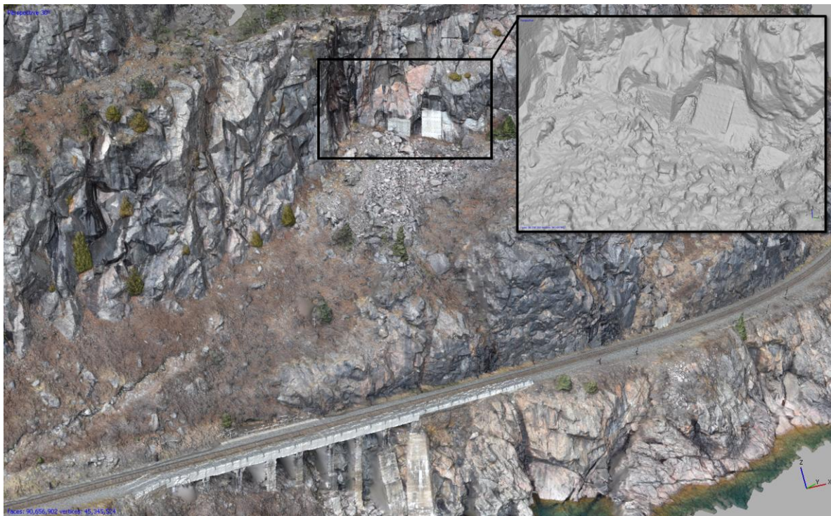
Figure 3. 3D model highlighting a practical level of detail achievable with OAP-H. Inset shows surface models of rock buttress, in which tie-back bolts are visible. CP Heron Bay Sub, Mile 72. Slope height approximately 100 m.
