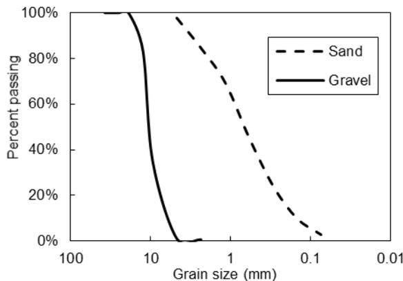
Figure 1. Size gradation of coarse and fine aggregates
