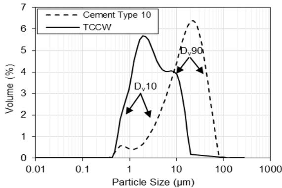
Figure 2. Particle size distribution based on volume percentage
