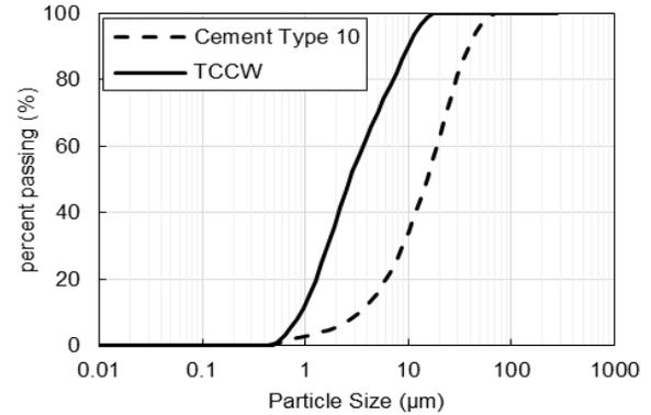
Figure 3. Particle size distribution of Thermo-mechanical cuttings cleaner waste and cement type 10
