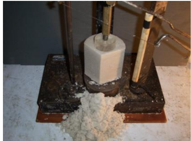
Figure 11: Stabilized Ottawa sand sample cut as stiff clay
