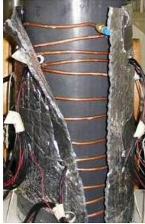
Figure 17: Laboratory setup used to simulate borehole end injection
