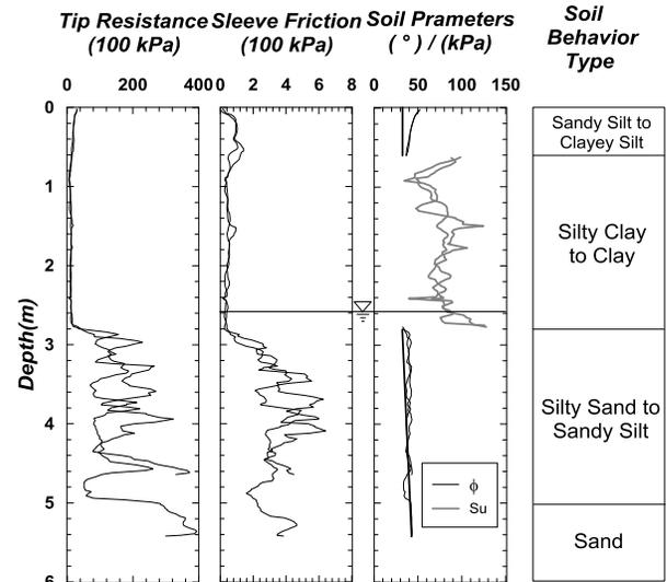
Figure 4. CPT profile of Site 3 at the Almita Yard in Ponoka
