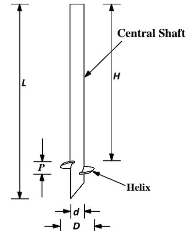
Figure 5. Sketch of tested single-helix pile
