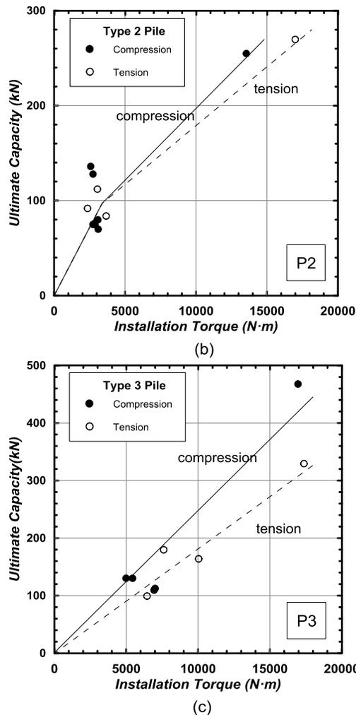
Figure 10. Torque factor design chart for tested piles
