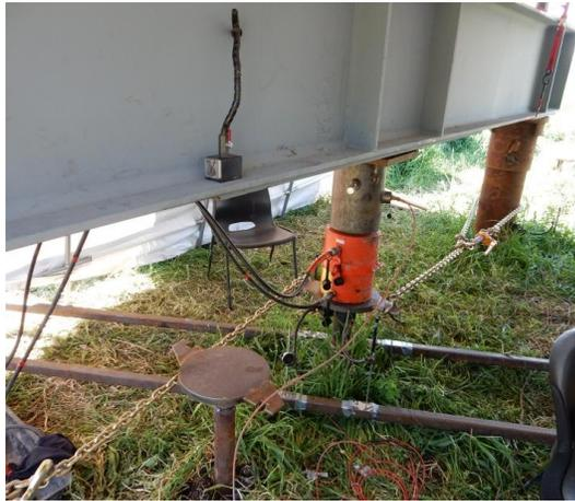
Figure 6. Setup of axial compression tests
