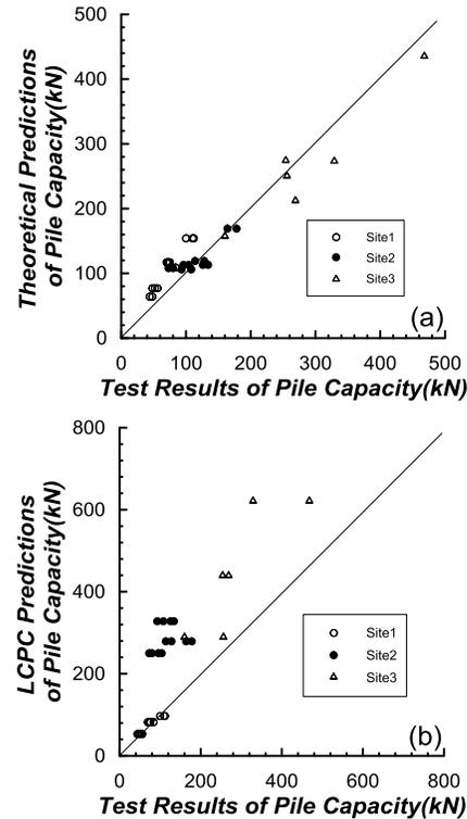
Figure 9. Comparison of predicted pile capacities and measured pile capacities using (a) theoretical method and (b) LCPC method
