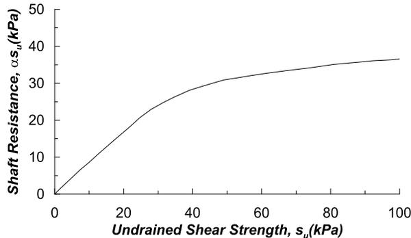
Figure 1. Adhesion ( $\alpha s_u$ ) of steel pile against undrained shear strength of clay (After Tomlinson 1957)
