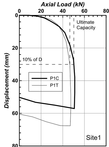
Figure 8 Load-Displacement curves of Type1 piles (P1) under compression (P1C) and tension (P1T) loading at Site1
