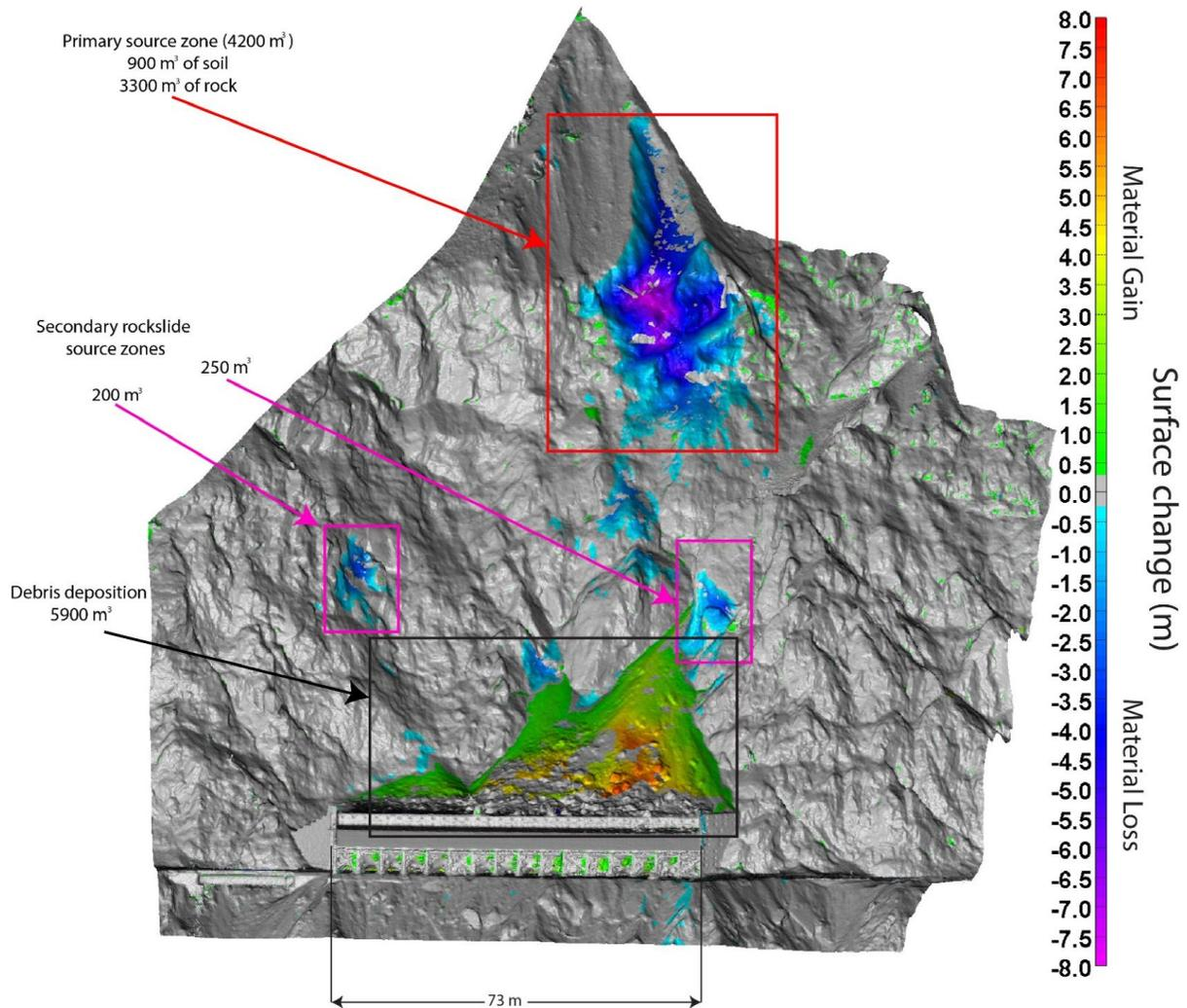
Figure 6. Shortest distance change detection 'isopach' model between the OAP data and the TLS data. Blue-purple colours indicate zones of material loss; green-red zones indicate zones of material gain.
