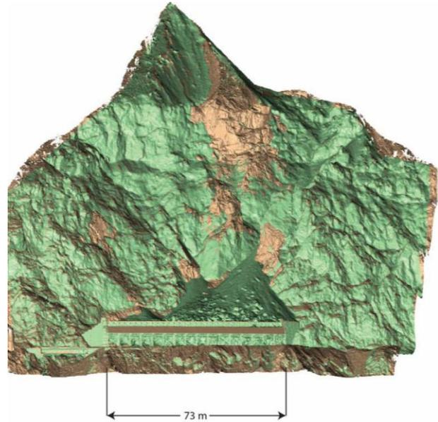
Figure 5. Visualization of the aligned 3D OAP surface model (green) to the TLS data (bronze).
