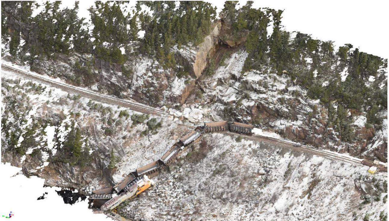
Figure 3. 3D photogrammetry point cloud model of the rock slide and train derailment site
