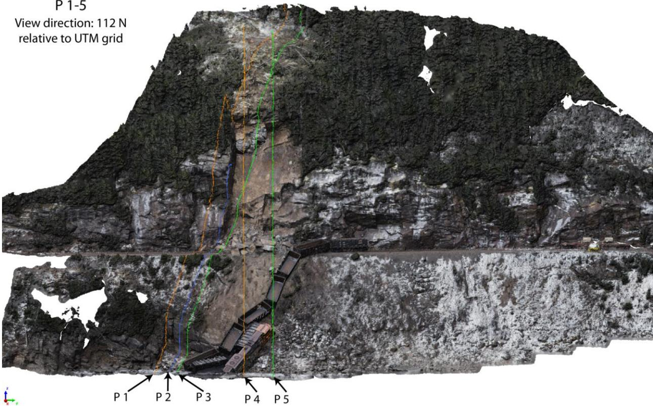
Figure 4. Annotated 3D surface model of the OAP with five profiles identified.
