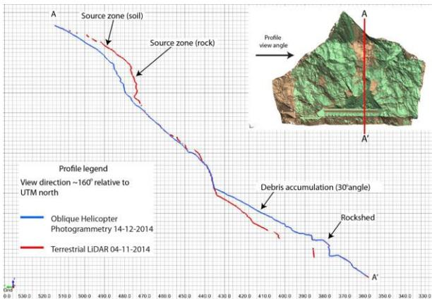
Figure 8. Profile perpendicular to the railway illustrating the pre failure slope topography (red) and the post failure slope topography (blue). Source and accumulation zones and identified in the figure.
