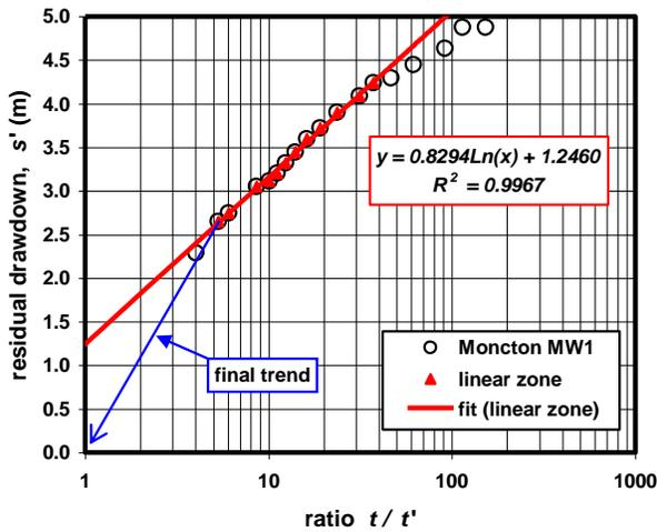
Figure 7. Graph of  $s'$  versus  $\log(t/t')$  for MW recovery data.
