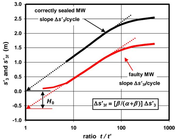
Figure 4. Graphs of  $s'_3$  and  $s'_{3f}$  versus  $\log t/t'$  for correctly sealed and faulty MWs.
