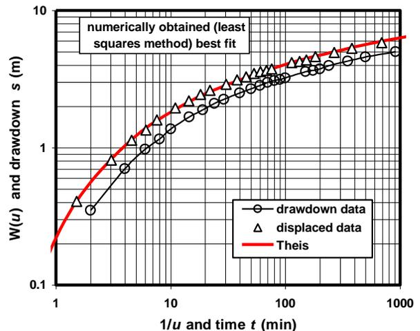
Figure 5: Method of Theis (1935) for MW drawdown data.
