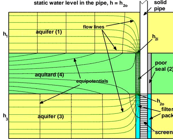
Figure 1. Schematic illustration of preferential seepage (hydraulic short-circuit) along a monitoring well (MW).
