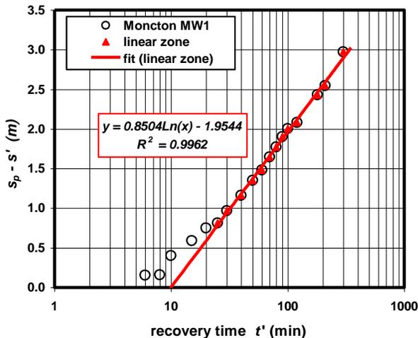
Figure 8. Graph of  $(s_p - s')$  vs.  $\log t'$  for MW recovery data.
