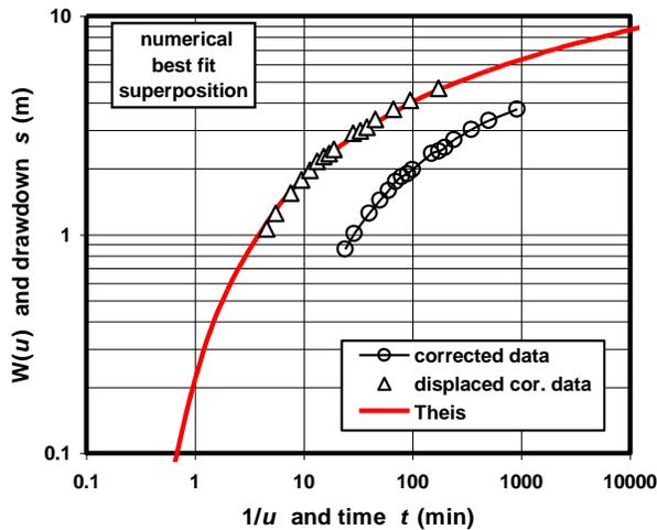
Figure 9. Method of Theis (1935) for corrected drawdown data of the monitoring well (MW).
