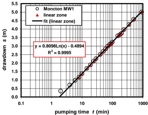
Figure 6. Method of Cooper-Jacob (1946) for MW drawdown data.
