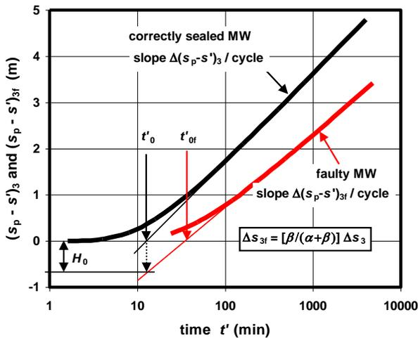
Figure 3. Graph of  $(s_p - s')_3$  and  $(s_p - s')_{3f}$  versus  $\log t'$  for correctly sealed and faulty MWs.
