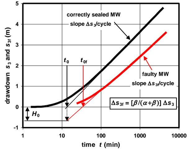
Figure 2. Graphs of  $s_3$  and  $s_{3f}$  versus  $\log(t)$  for correctly sealed and faulty monitoring wells.
