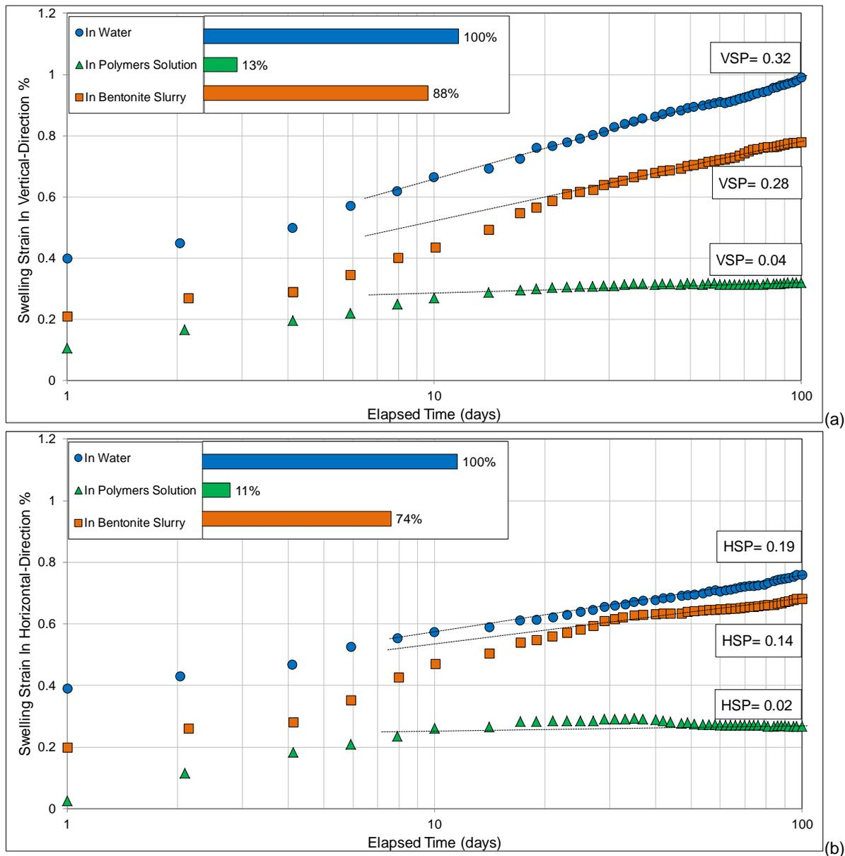
Figure 2. Typical results of the free swell tests performed on Niagara Queenston shale from depth  $\approx$ 125 m-137 m below natural ground level: a) Vertical strains, b) Horizontal strains
