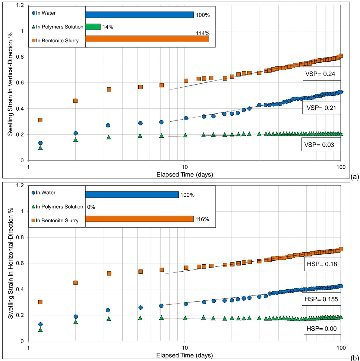
Figure 3. Typical results of the free swell tests performed on Milton Queenston shale from depth  $\approx$ 18 m-33 m below natural ground level: a) Vertical strains, b) Horizontal strains
