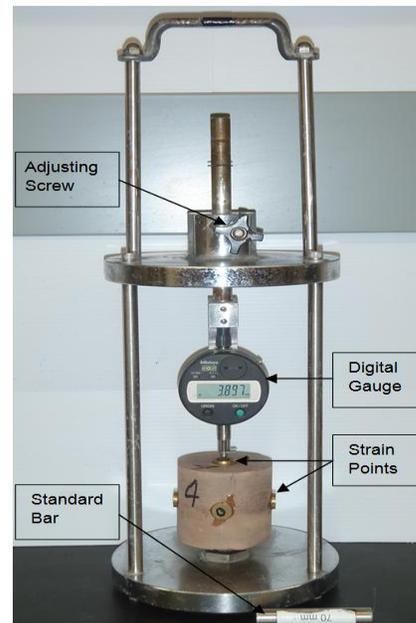
Figure 1. Free swell test apparatus and specimen
