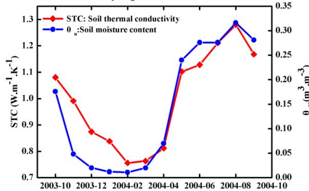
Figure 2 Effect of soil moisture content on thermal conductivity
