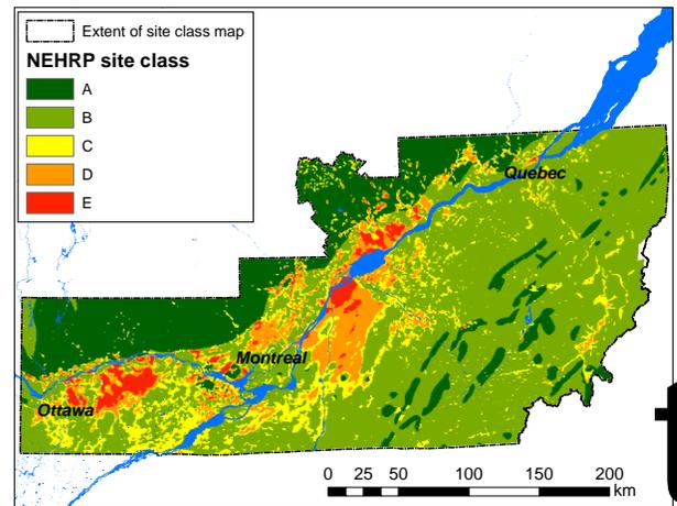
Figure 3. Site Class for the western half of the study area inferred from 3D Geological Model (Nastev et al. 2014)
