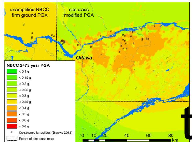
Figure 7. Ottawa area dated large landslides and amplified 2475 year PGA
