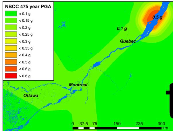
Figure 1. NBCC 10 % in 50 years (475 year) PGA for uniform firm ground (Site Class C)
