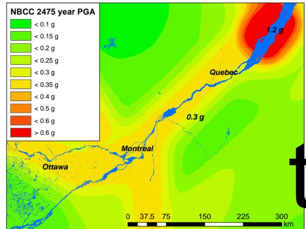
Figure 2. NBCC 2 % in 50 years (2475 year) PGA for uniform firm ground (Site Class C)
