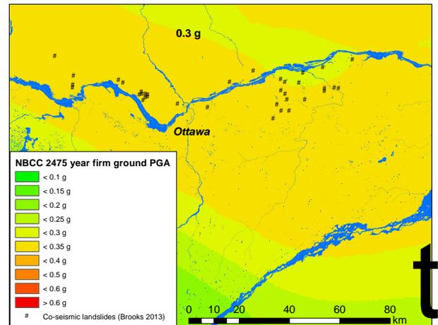
Figure 6. Ottawa area dated large landslides (from Brooks, 2013) and firm ground 2475-yr PGA.
