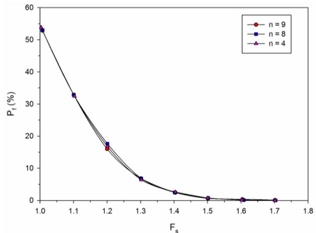
Figure 9. Effect of number of reinforcement layers on probability of internal failure mechanism
