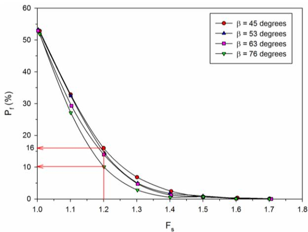
Figure 10. Effect of slope angle on probability of internal failure mechanism
