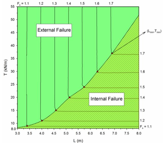
Figure 4. Contour plot for  $F_s$  values corresponding to internal and external failure mechanisms for  $\beta = 45$  degrees and  $n = 4$  reinforcement layers
