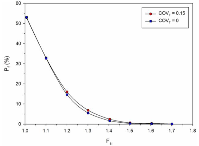
Figure 8. Effect of constant tensile strength ( $COV_T = 0$ ) and random variability in reinforcement tensile strength ( $COV_T = 0.15$ ) on the probability of internal failure mechanism
