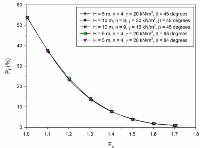
Figure 6. Probability of external failure mechanism versus factor of safety for different slope angles and  $n = 4$
