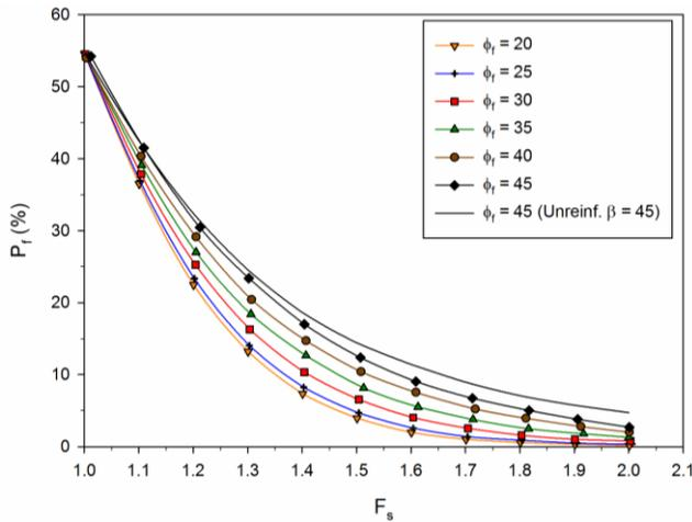
Figure 7. Probabilistic slope stability chart for different values of  $\phi_f$  to generate external failure mechanism
