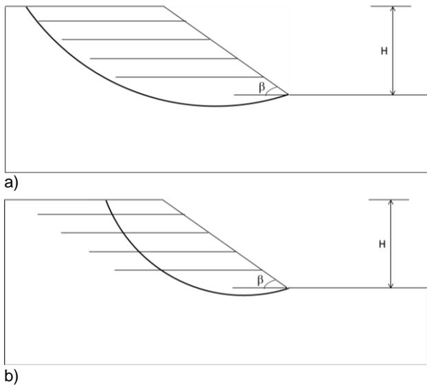
Figure 1. a) External failure mechanism, b) Internal failure mechanism
