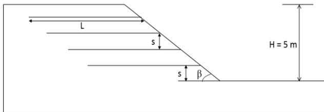
Figure 2. Example slope with four layers of geosynthetic reinforcement ( $n = 4$ ) and  $H = 5$  m
