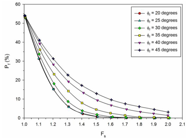
Figure 11. Probabilistic slope stability chart for reinforced soil slopes with internal failure mechanisms and different values of  $\phi_r$  ( $\beta = 45$  degrees)
