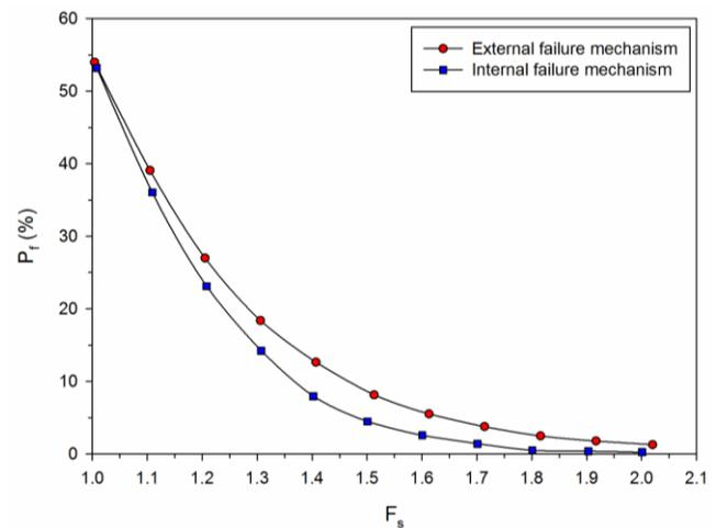
Figure 12. Difference between probabilities of failure in external failure mechanism and internal failure mechanism for the same mean value of  $F_s$  and for  $\phi_r = 35$  degrees
