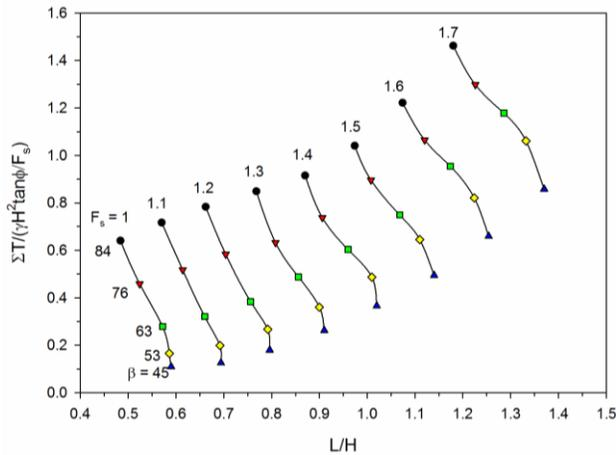
Figure 5. Minimum normalized reinforcement tensile strength versus minimum normalized reinforcement length to generate only external failure mechanisms for reinforced slopes with  $n = 4$  reinforcement layers
