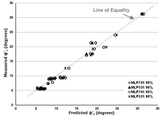
Figure 4. The predicted and measured  $\phi_r$  comparison for all models; Stark and Hussain (2013) test dataset.
