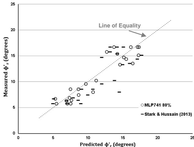
Figure 5. The measured and predicted  $\phi'_r$  for Clifton data from the MLP741 80% model and Stark and Hussain (2013) empirical method.
