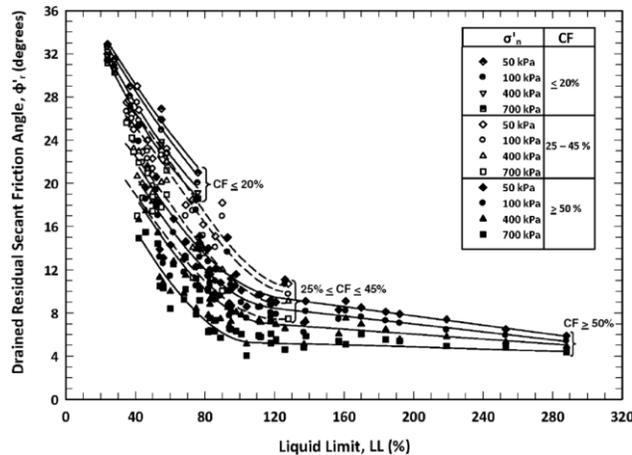
Figure 1. Empirical correlation for  $\phi'_r$  angle based on LL, CF, and normal stress (Stark and Hussain 2013)
