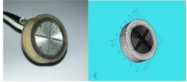
Fig. 3. Actual and simulated piezoelectric sensor.
