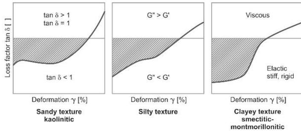
Figure 9: General shape of the  $\tan(\delta)$  versus strain according to the soil texture (Markgraf et al.)
