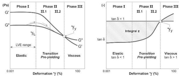
Figure 6: Storage modulus ( $G'$ ) and loss modulus ( $G''$ ) in the left ;  $\tan(\delta)$  in the right (Markgraf et al. 2012)
