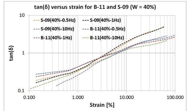
Figure 11:  $\tan(\delta)$  versus strain for B-11 and S-09 ( $W = 40\%$ )
