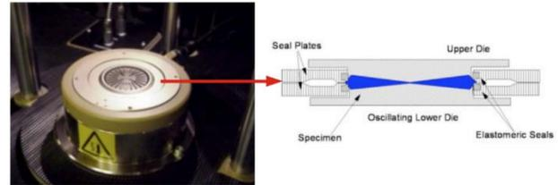
Figure 8 : Lower plate of the SIS-V50 rheometer - Section of the closed rheometer
