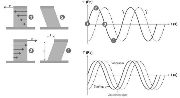
Figure 4: Principles of sinusoidal strain measurements (Markgraf and Horn)
