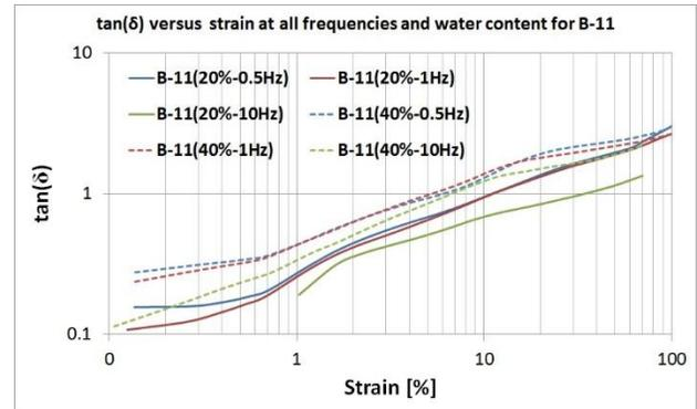
Figure 13:  $\tan(\delta)$  versus strain at all frequencies and water content for B-11
