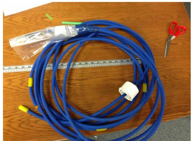
Figure 10. Each of the thermistor strings are prepared for insertion by protecting the exposed wiring, and locking the PVC cap into the correct position.
