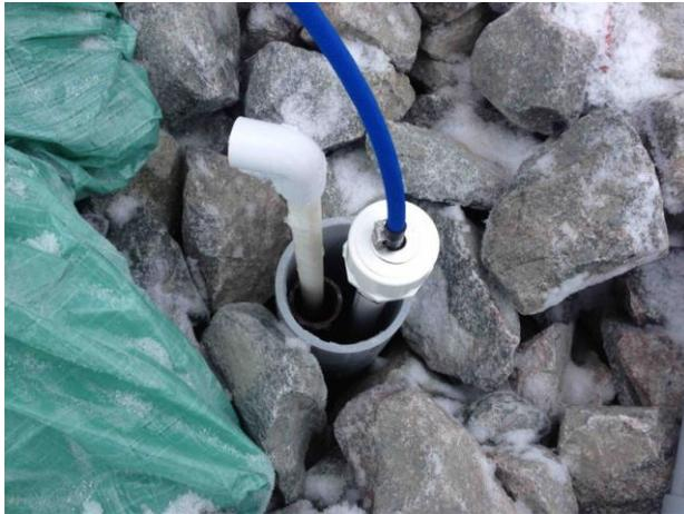
Figure 11. The thermistor string is fed into the PEX pipe, alongside the steel convection pipe.
