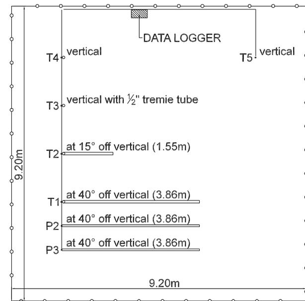
Figure 16. Plan view of the field monitoring program site.
