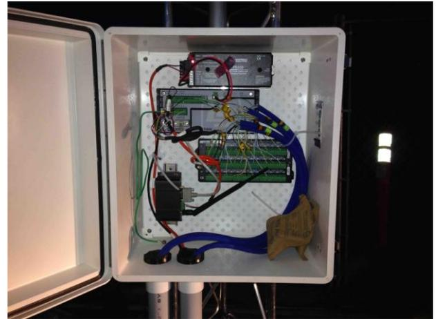
Figure 14. All thermistor strings feed into the datalogger contained in a fiberglass enclosure on site.
