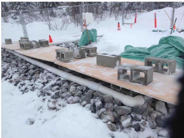
Figure 13. A plywood roof is constructed over the system to protect against precipitation entering the convection pipes during testing.
