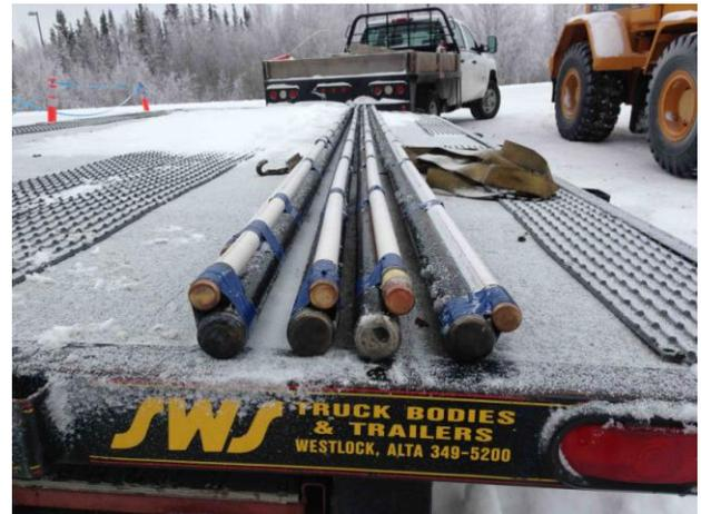
Figure 4. PEX pipes to contain the thermistor strings are attached to the 6 m long steel pipes.
