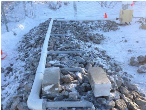
Figure 12. The white PVC manifold contains and protects the thermistor strings.
