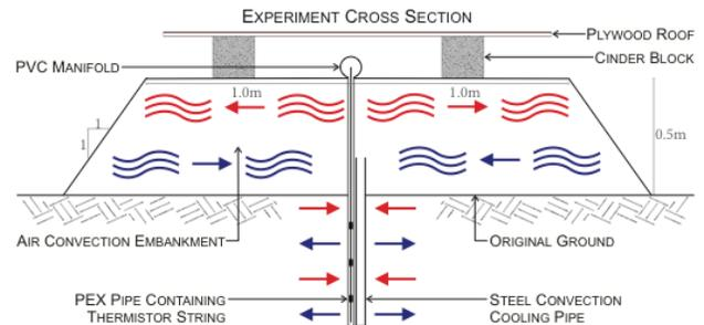
Figure 15. Experiment cross section at point T4.
