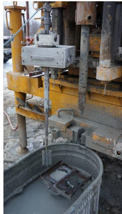
Figure 1. Up-hole torque motor holding downhole vane load cell and rectangular (150mm by 75 mm) vane over mud-rotary supported borehole at Gloucester, ON
