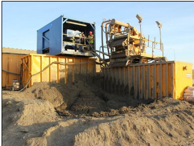
Figure 4.2 - Typical 3 stage solids separation system
