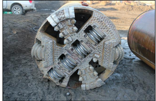
Figure 4.1 - Herrenknecht AVN1200TC with mixed ground cutting wheel attached
