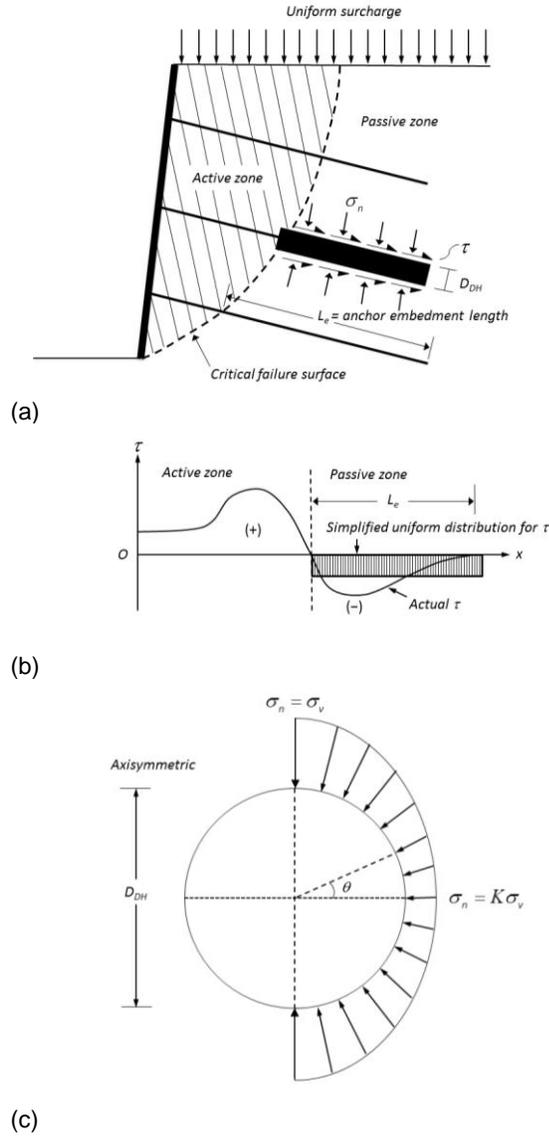
Fig. 1. Nail pullout limit state: (a) soil nail wall; (b) shear stress along a soil nail; (c) cross-sectional view showing normal stress acting on grouted soil nail
