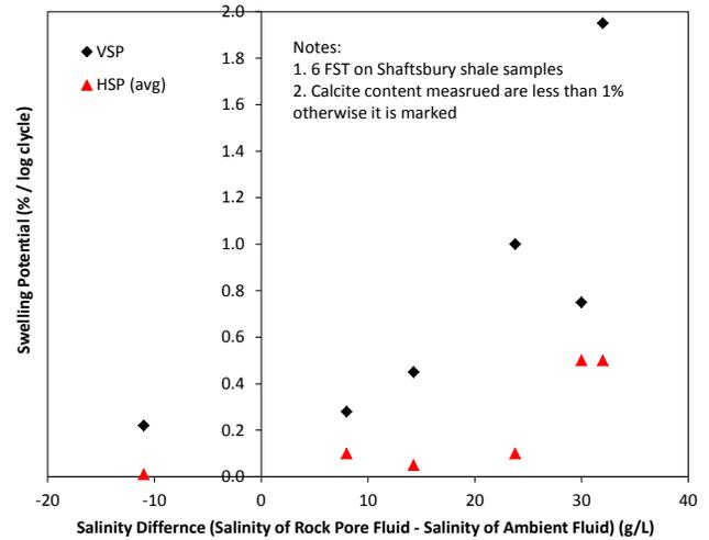
Figure 6. Swelling potential versus salinity difference from salinity of rock pore fluid to salinity of ambient fluid on Shaftesbury shale
