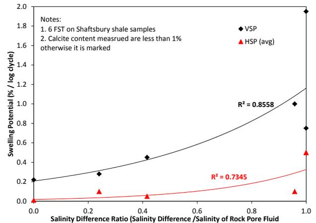
Figure 7. Swelling potential versus salinity difference from salinity of rock pore fluid to salinity of ambient fluid on Shaftesbury shale
