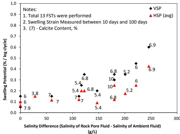
Figure 2. Swelling potential versus salinity difference from salinity of rock pore fluid to salinity of ambient fluid on Queenston shale
