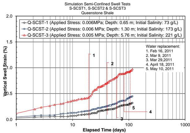
Figure 8. Result of SCSTs on Queenston shale with replacement of ambient fluid during tests
