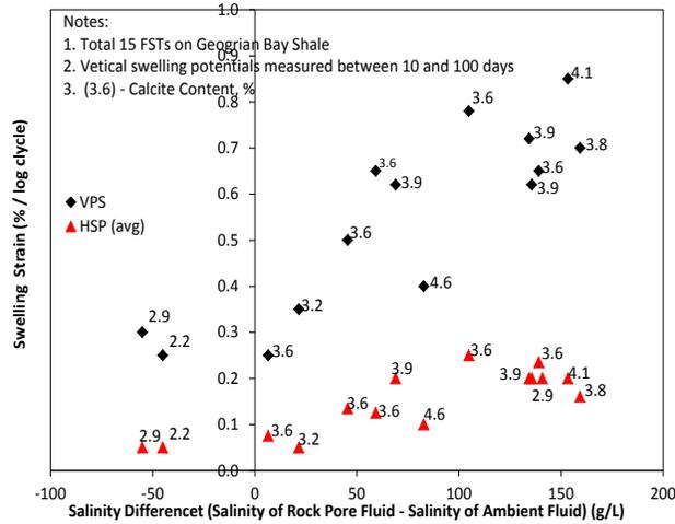
Figure 4. Swelling potential versus salinity difference from salinity of rock pore fluid to salinity of ambient fluid on Georgian Bay shale
