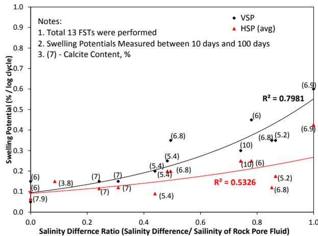
Figure 3. Swelling potential versus salinity difference ratio on Queenston shale
