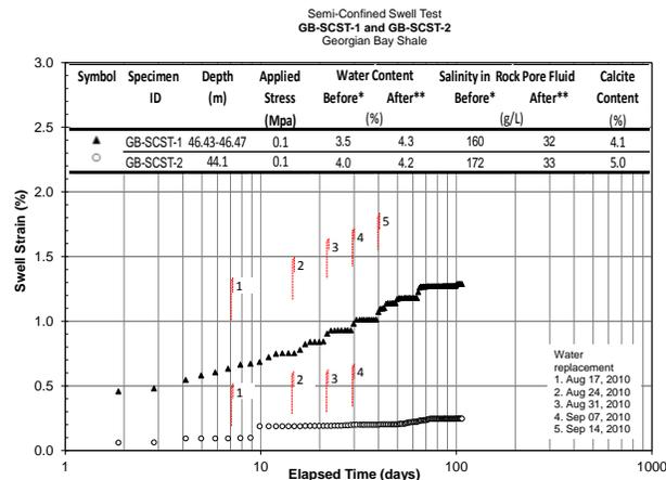
Figure 9. Result of SCSTs on Georgian Bay shale with replacement of ambient fluid during tests.
