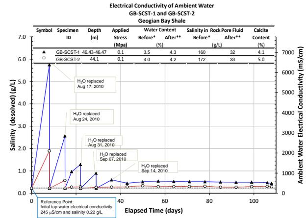
Figure 10. Salinity measurements of ambient fluid during SCSTs on Georgian Bay shale
