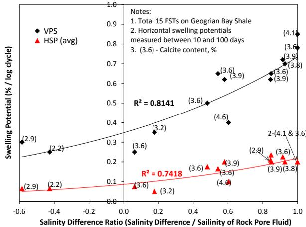
Figure 5. Swelling potential versus salinity difference ratio on Georgian Bay shale
