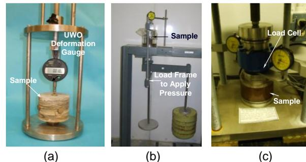
Figure 1. Typical setup of swell tests: (a) FST, (b) SCST and (c) NST
