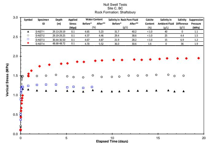
Figure 11. Results of NST with difference salt concentrated ambient fluid.
