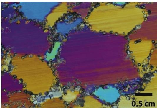
Figure 7. Ice sample viewed under cross-polarized light.
