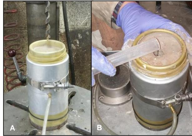
Figure 3: Hydrate vein formation within soil
