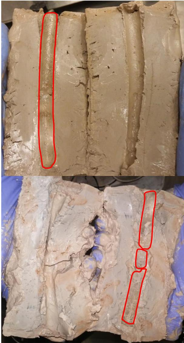
Figure 5: Laboratory-formed hydrate veins (outlined in red) within soil after (A) being kept within the stability field ( $<2.15^{\circ}\text{C}$ ) for 24 hours and (B) kept at a cell pressure of 500 kPa with no effective stress for 24 hours.
