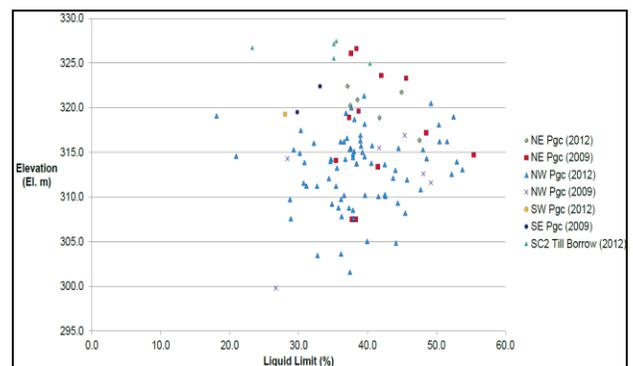
Figure 10: Distribution of liquid limits with elevation and location within SZ2
