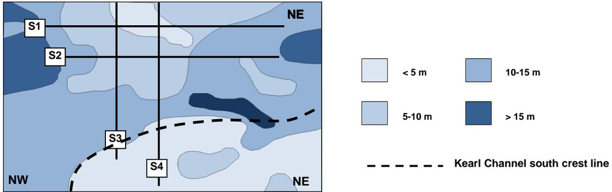
Figure 8: Isopach showing the thickness of the moraine assemblage within SZ2. Based on 119 boreholes from the study area
