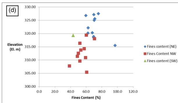
Figure 8: Distribution of (a) Sand content (b) Silt content (c) clay content (d) fines contents with elevation and location within the glacial tills within SZ2
