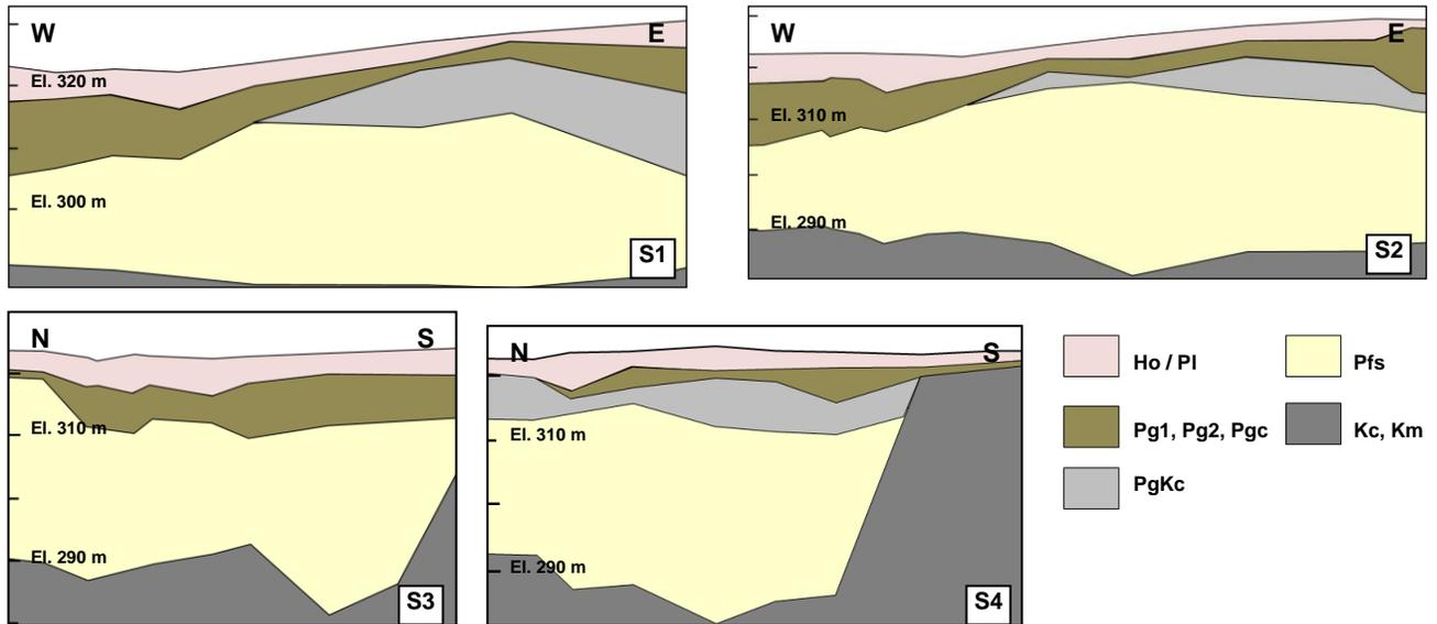
Figure 9: Schematic cross-sections through the moraine assemblage within SZ2
