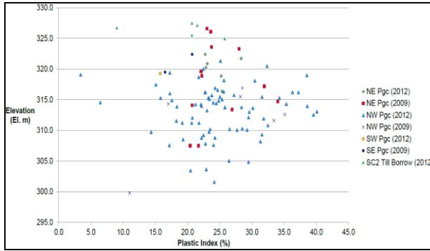
Figure 11: Distribution of plastic index with elevation and location within SZ2
