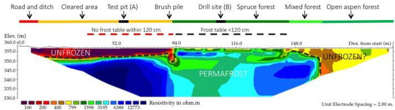
Figure 6. 200 m-long resistivity profile running across a cleared field and into a relatively undisturbed forest in the Dawson City region. The boundary between frozen and unfrozen materials (dashed line) is interpreted to be at about 800 Ohm m (between the yellow and green shades).
