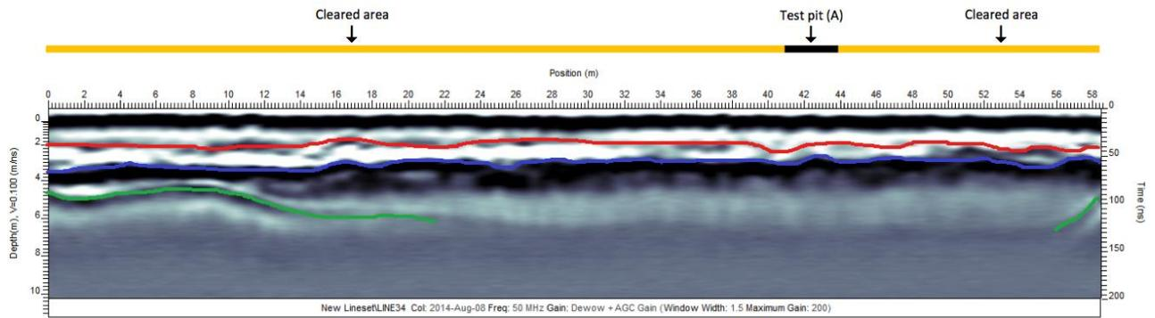
Figure 5. 59 m-long GPR profile A conducted in a cleared field in the Dawson City region. Survey had a penetration depth of 7 m at a speed of 0.1 m/ns. Stratigraphic contacts are present at 2 m (red line), 4 m (blue line) and 5-7 m (green line).
