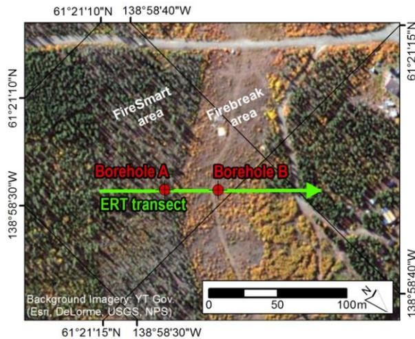
Figure 2. View of the FireSmart zone and firebreak in Burwash Landing. Green line represents ERT transect; red dots represent borehole locations.
