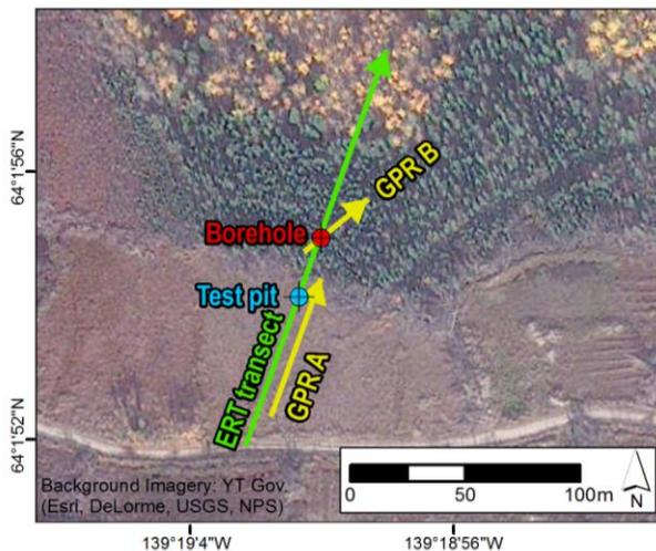
Figure 4. Semi-cleared placer-mining claim (image date: 2012) showing locations of geophysics profiles and boreholes in cleared field and forested area.
