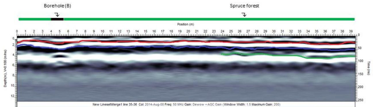
Figure 7. 40 m-long GPR profile B conducted in a forest in the Dawson City region. Survey had a penetration depth of 6 m at a speed of 0.1 m/ns. Stratigraphic contacts are present at 0.5-1 m (red line), 2 m (blue line) and 4-6 m (green line).
