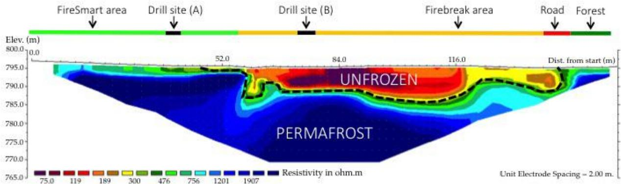
Figure 3. 160 m-long resistivity profile covering the FireSmart zone, the firebreak, a gravel road, and a portion of relatively undisturbed forest in Burwash Landing, YT. The boundary between frozen and unfrozen materials (dashed line) is interpreted to be at about 300 Ohm m (between the yellow and green shades).
