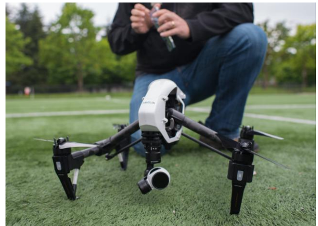
Figure 1. Photograph of the DJI Inspire 1 UAV prepared for take-off. Note the camera attached by a 3-axis gimbal on the front of the UAV.
