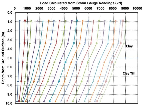
Figure 8 Load distribution along test pile at Site 1
