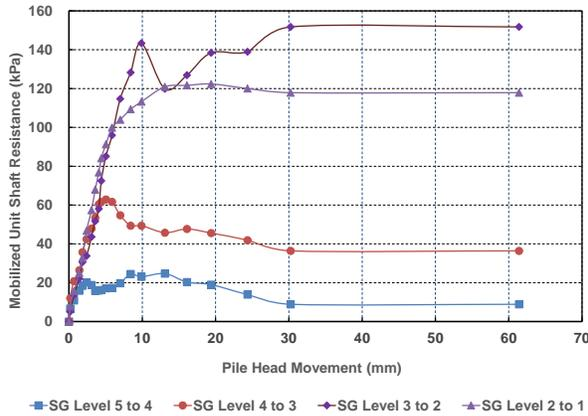
Figure 13 Mobilized unit shaft resistance from pile loading test at Site 3
