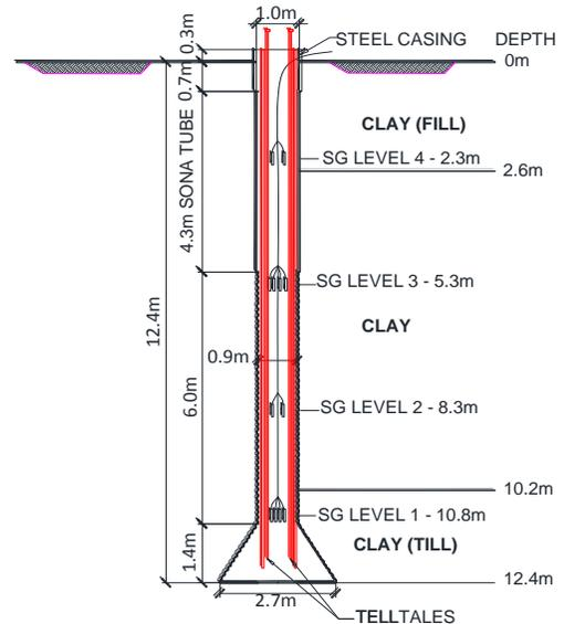
Figure 3 Schematic section of test pile at site 2
