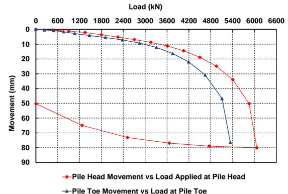
Figure 6 Load displacement curve for test pile at Site 2
