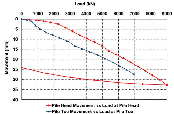
Figure 5 Load displacement curve for test pile at Site 1
