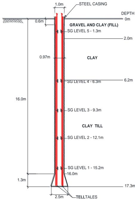
Figure 4 Schematic section of test pile at Site 3
