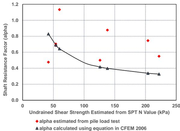
Figure 14 Shaft resistance coefficient vs undrained shear strength
