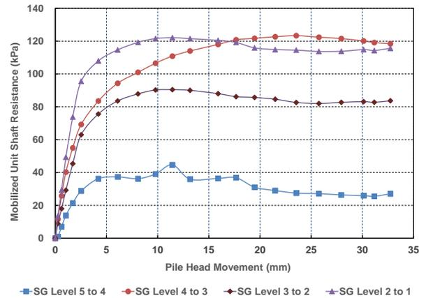
Figure 11 Mobilized unit shaft resistance from pile loading test at Site 1
