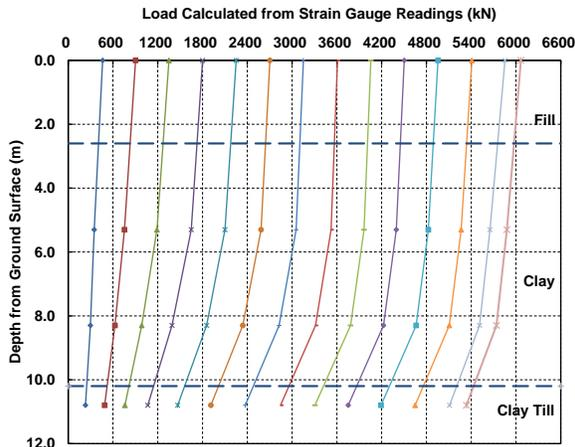
Figure 9 Load distribution along test pile at Site 2
