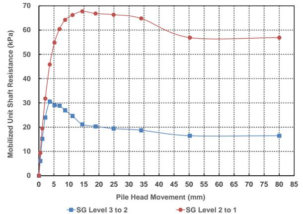
Figure 12 Mobilized unit shaft resistance from pile loading test at Site 2
