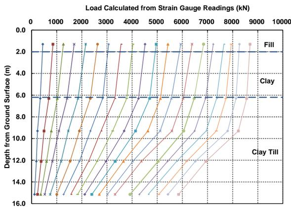
Figure 10 Load distribution along test pile at Site 3
