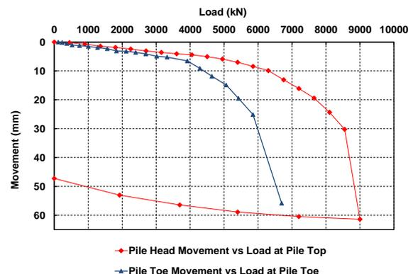
Figure 7 Load displacement curve for test pile at Site 3
