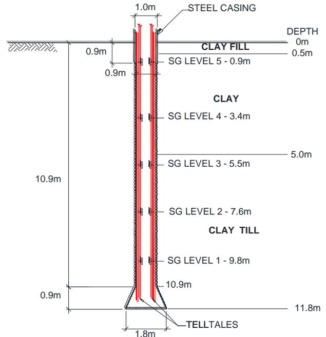
Figure 2 Schematic section of test pile at Site 1
