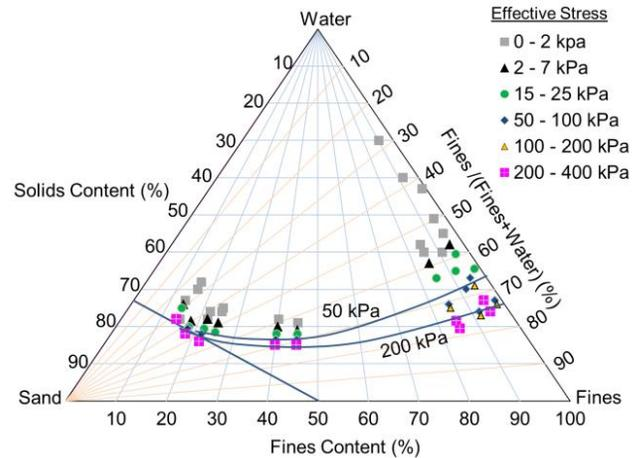
Figure 11. Compressibility of different oil sands tailings
