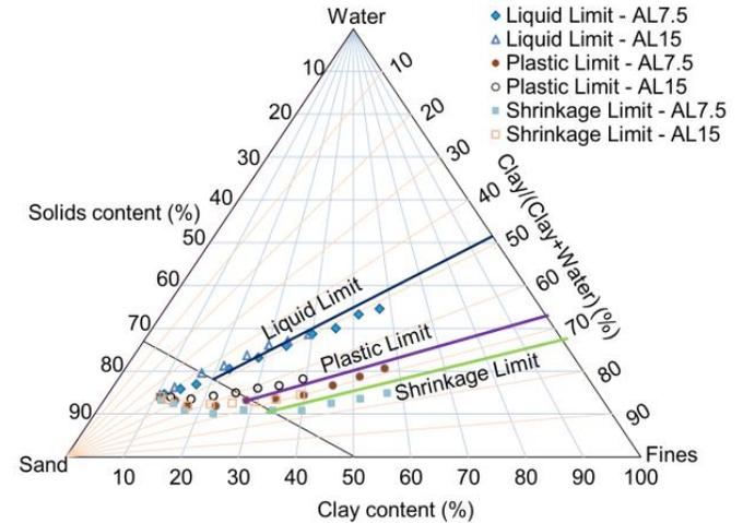
Figure 8. Atterberg limits as a function of CWR
