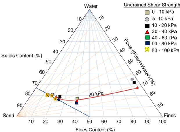
Figure 14. Undrained shear strength of different oil sands tailings
