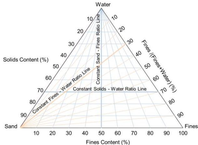
Figure 4. The Soil Structure Behaviour Diagram
