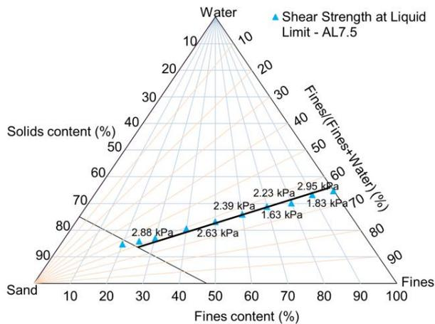
Figure 13. Shear strength at liquid limit (after Sorta et al. 2012)
