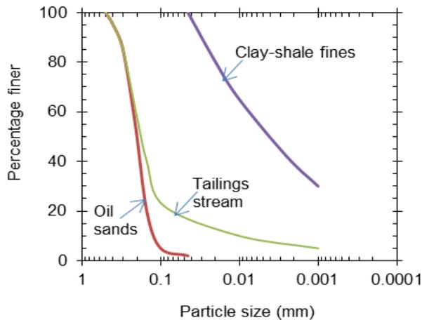
Figure 2. PSD of oil sands ore, clay-shale inclusions and resulting tailings stream
