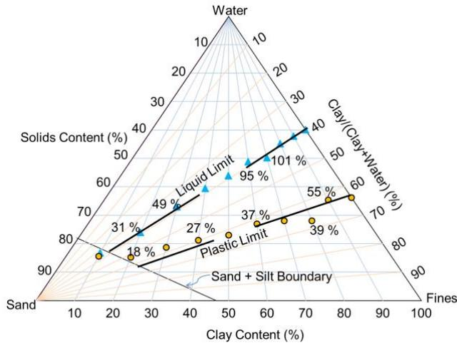
Figure 9. Atterberg limits for Middle East sand and clay mixtures (after Azam 2003)
