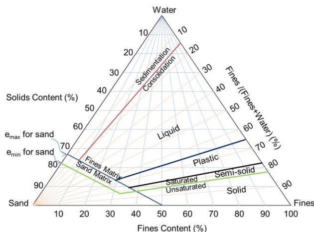
Figure 5. Typical characteristics of oil sands tailings
