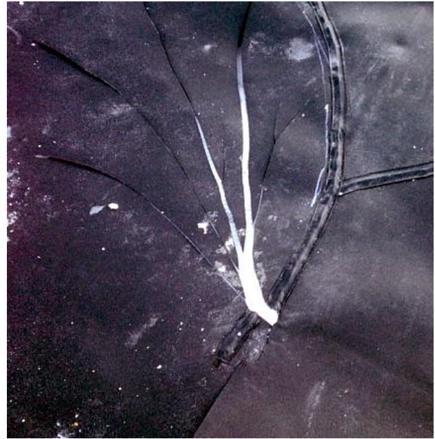
Figure 7. Cracking of the geomembrane.
