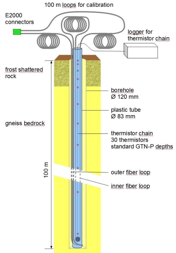
Figure 2. The borehole equipment.
