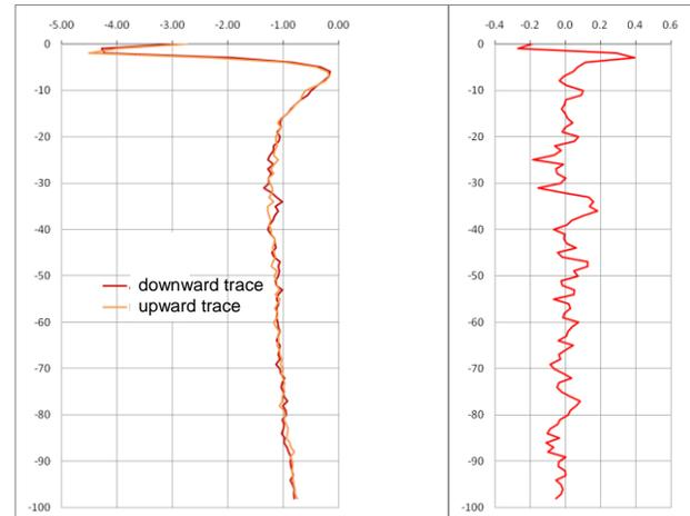
Figure 3. DTS measurements of January 2013. Left: downward and upward temperature profiles. Right: difference between the two profiles.
