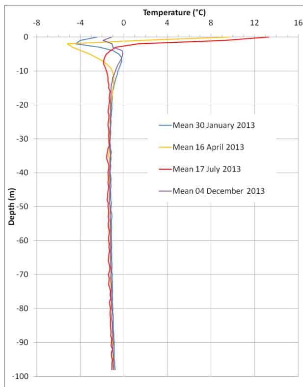
Figure 4. Averaged temperature profiles at the four measurement dates. Each profile is the mean of 4 single traces.
