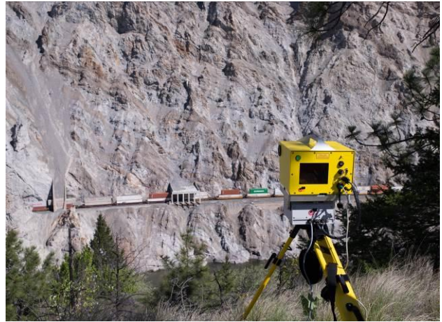
Figure 1: TLS setup in the White Canyon, approximately 350 m from the railway track.
